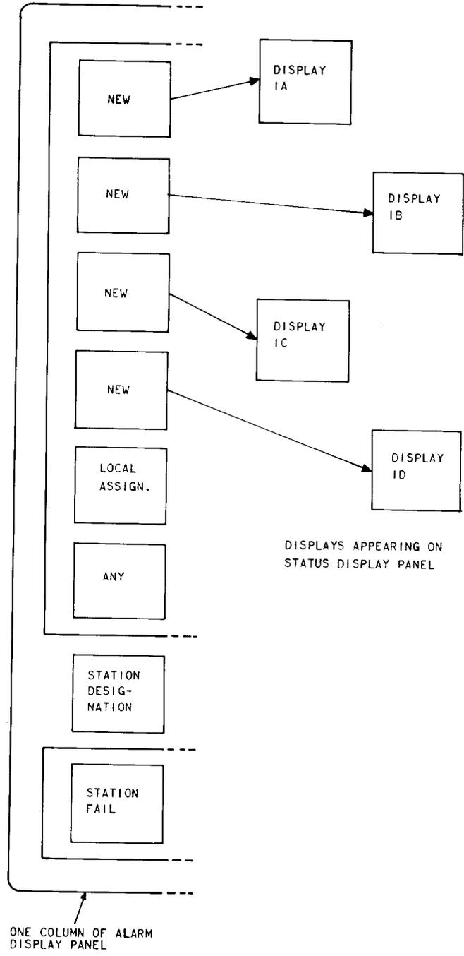
Fig. 5—Alarm Display for E2 Systems in Which All Stations Have Four Status Displays (New Assignment Philosophy)
