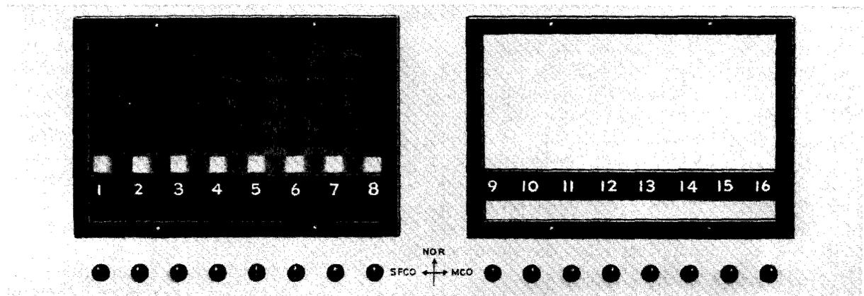
Fig. 2—Typical Alarm Display Panel
