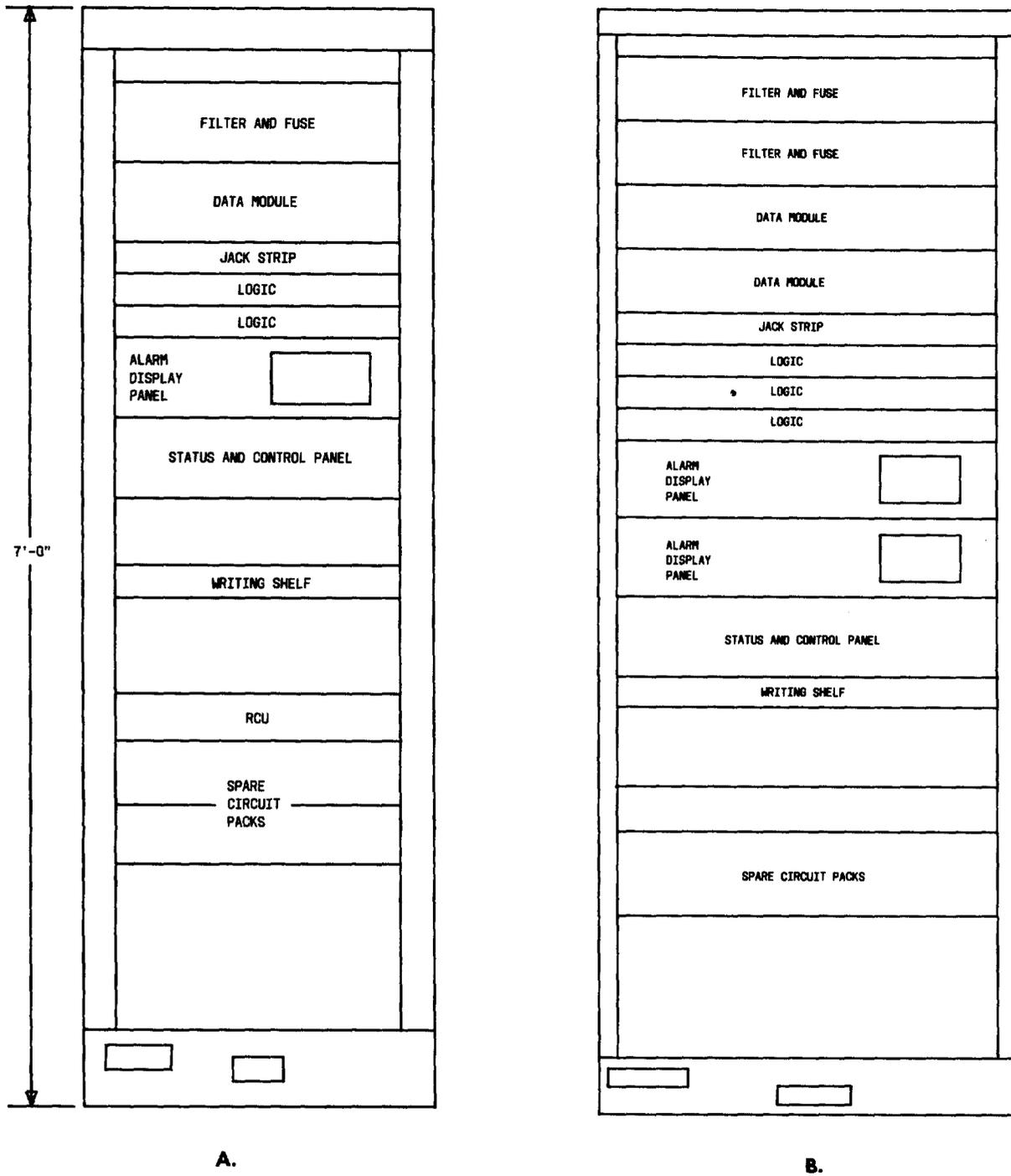
Fig. 1—Typical Manual Alarm Central (J92617)
