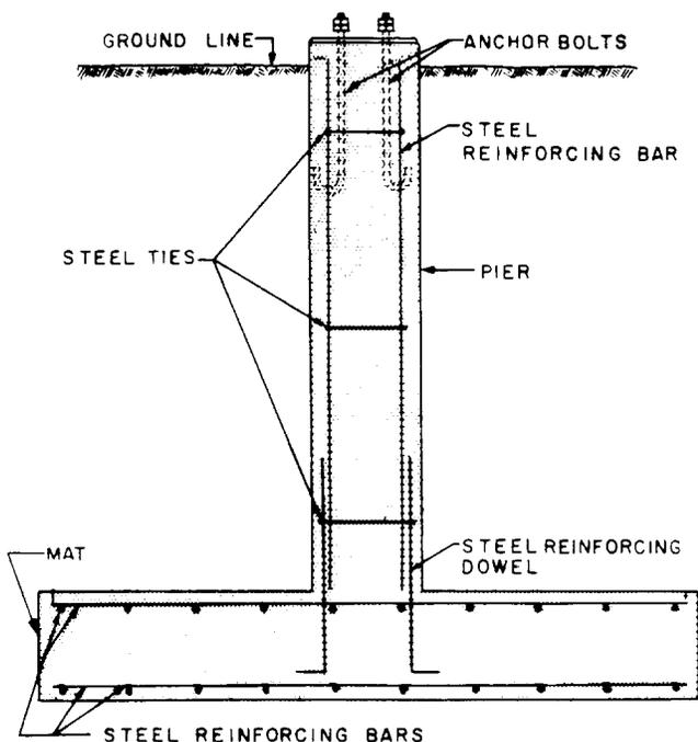
Fig. 1—Cross-Sectional View of Typical Foundation Pier and Mat for One Leg of Self-Supporting Towers
