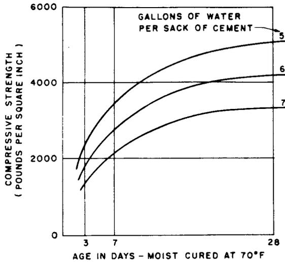
FIG. A NORMAL PORTLAND CEMENT CONCRETE
