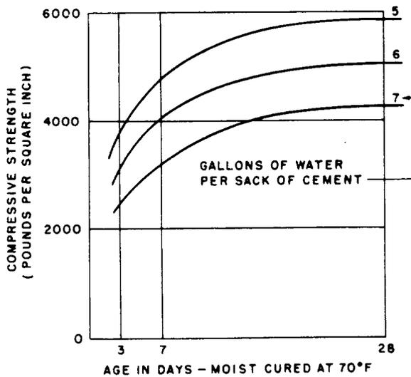
FIG. B HIGH-EARLY STRENGTH PORTLAND CEMENT CONCRETE
