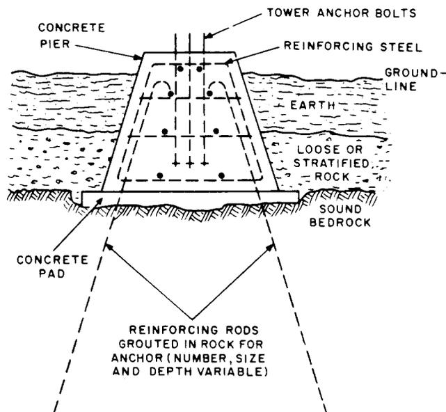
Fig. 3—Typical Foundation in Rock
