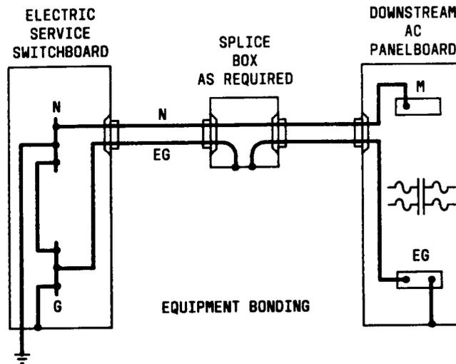
Fig. 3—Equipment Bonding
