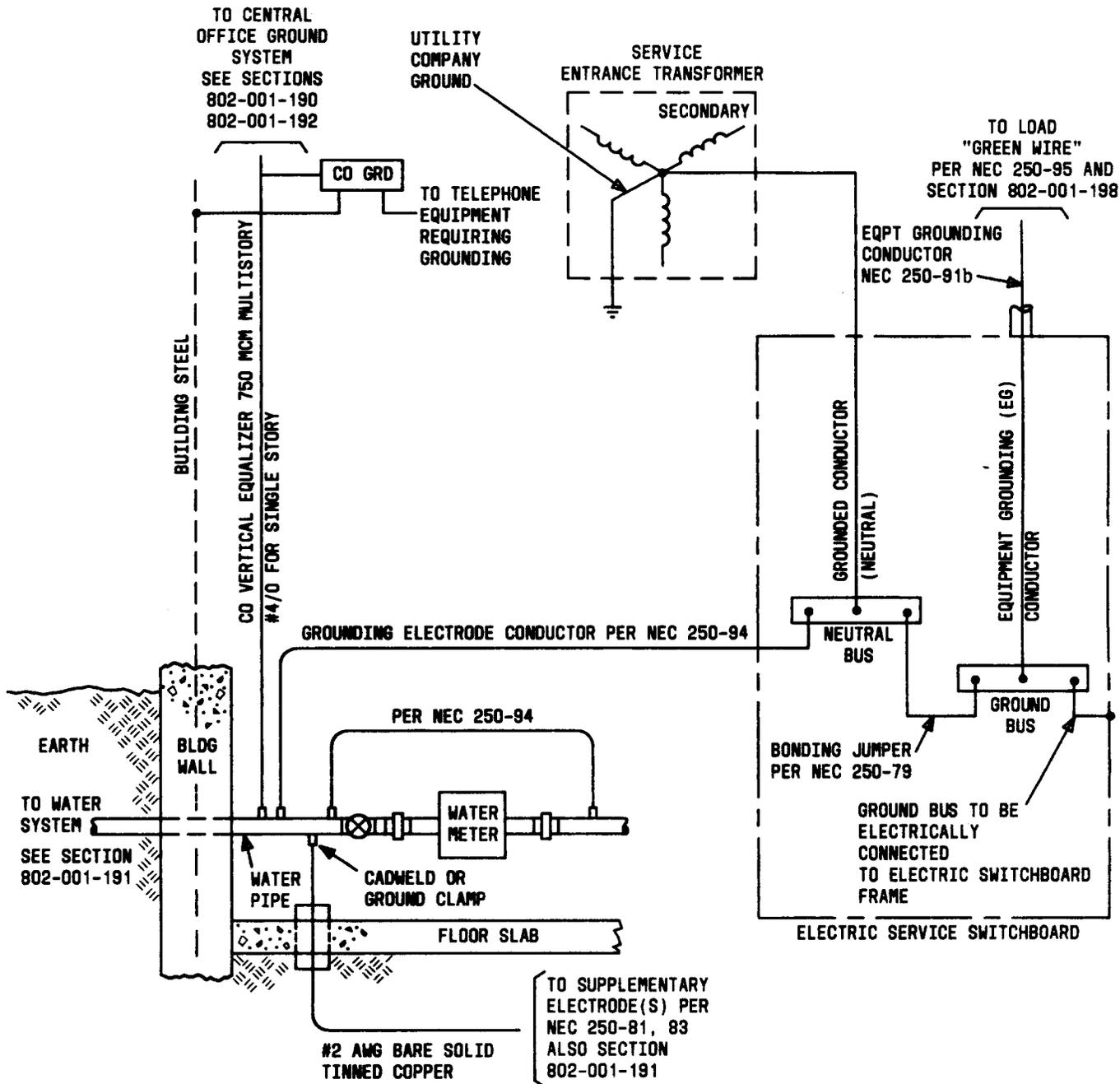
Fig. 1 — Typical Grounding Schematic
