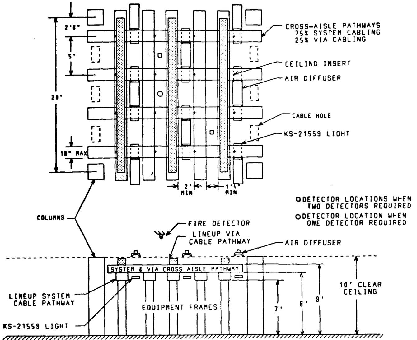
Fig. 2—Cable Pathways Plan for 7- to 10-Foot Space
