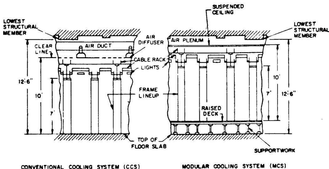
Fig. 1—Typical Equipment Frame Areas
