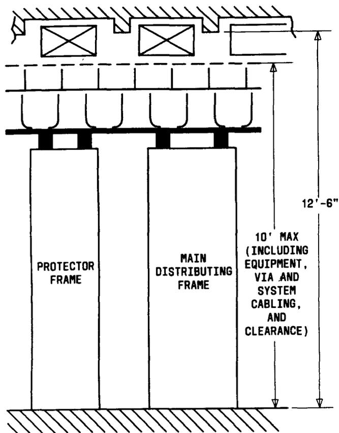
Fig. 4—Typical Distributing Frame Area
