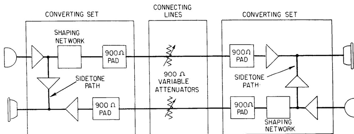
FIG. 13—LABORATORY BASIC TELEPHONE CONNECTION
