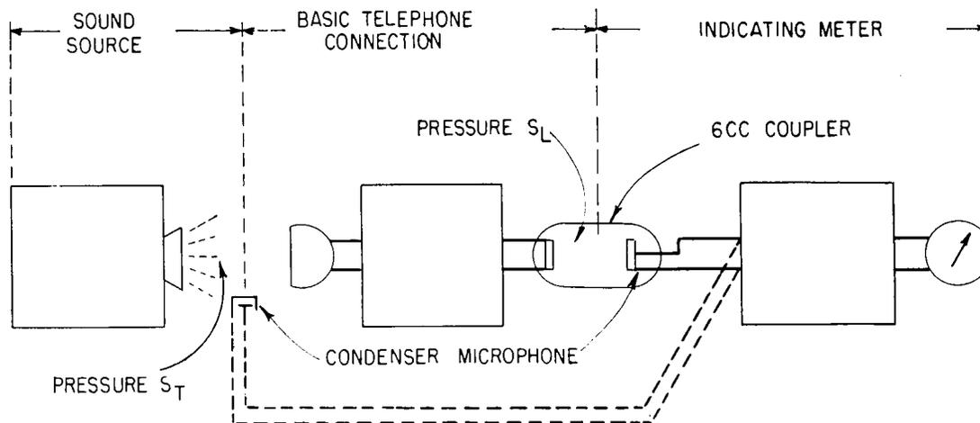
FIG. 9—ELECTRO-ACOUSTIC TRANSMISSION MEASURING SYSTEM
