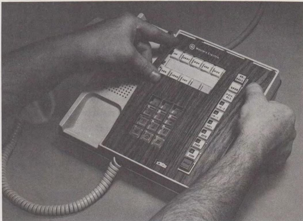
**Fig. 11—Replacing Faceplate**
