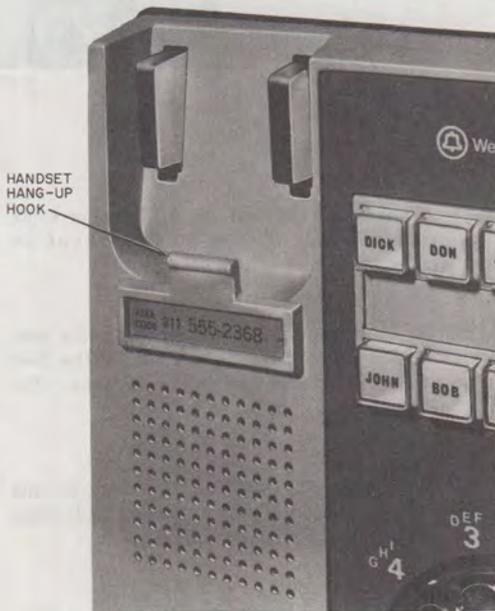
Fig. 9—Handset Hook Attachment for Wall Set
