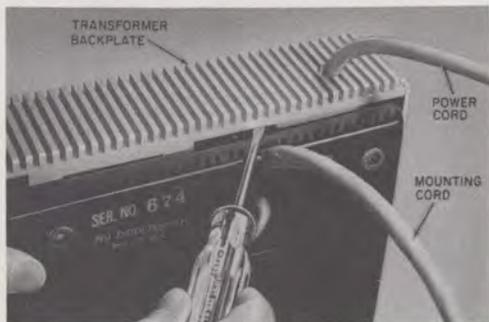
Fig. 5—Removing Transformer
