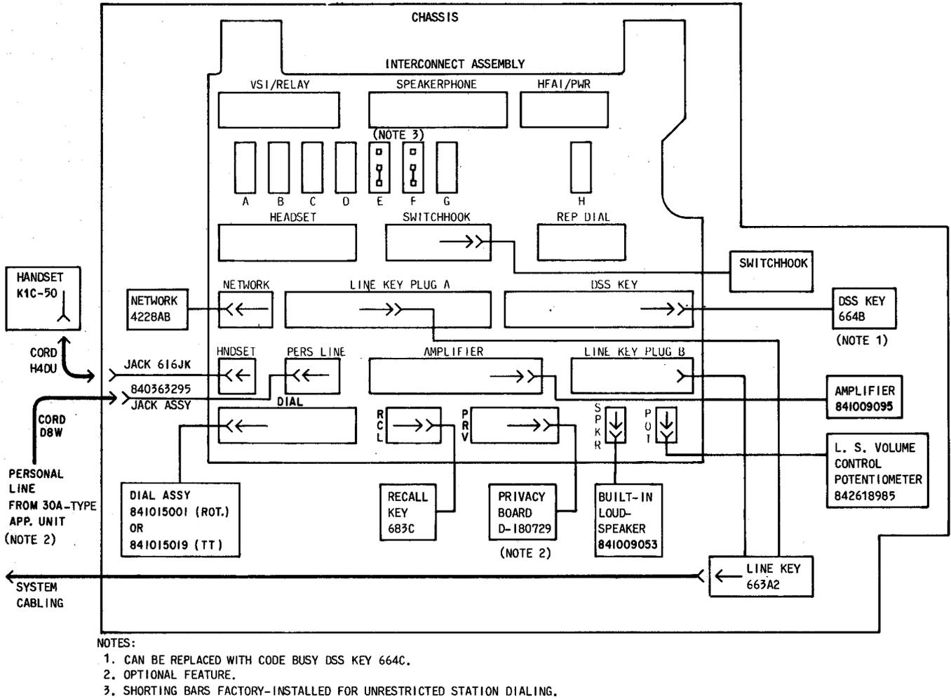
Fig. 50—Block Diagram of Basic Satellite Wall Set
