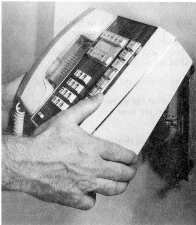
**Fig. 18—Mounting Wall Set on Wall Plate**
