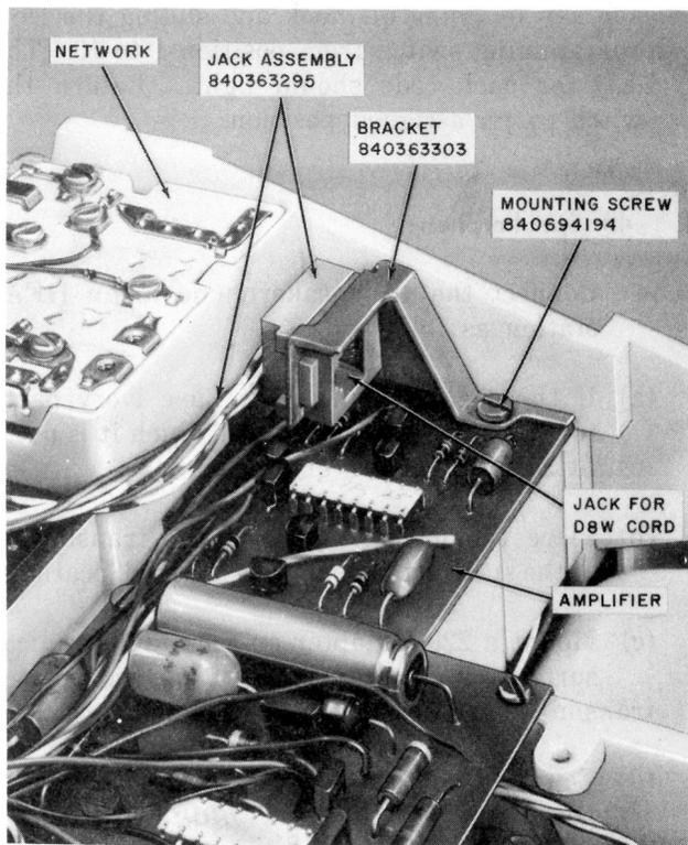
**Fig. 41—Installation of Personal Line Jack Assembly**
