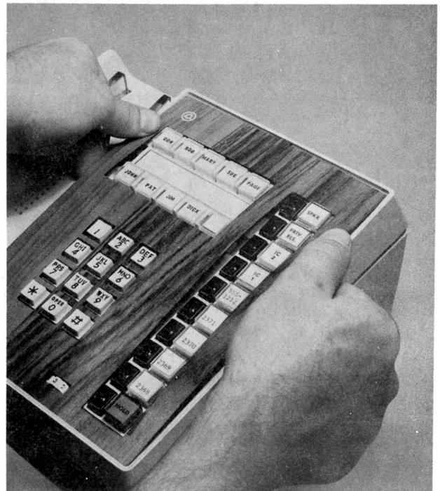
Fig. 54—Installing Faceplate
