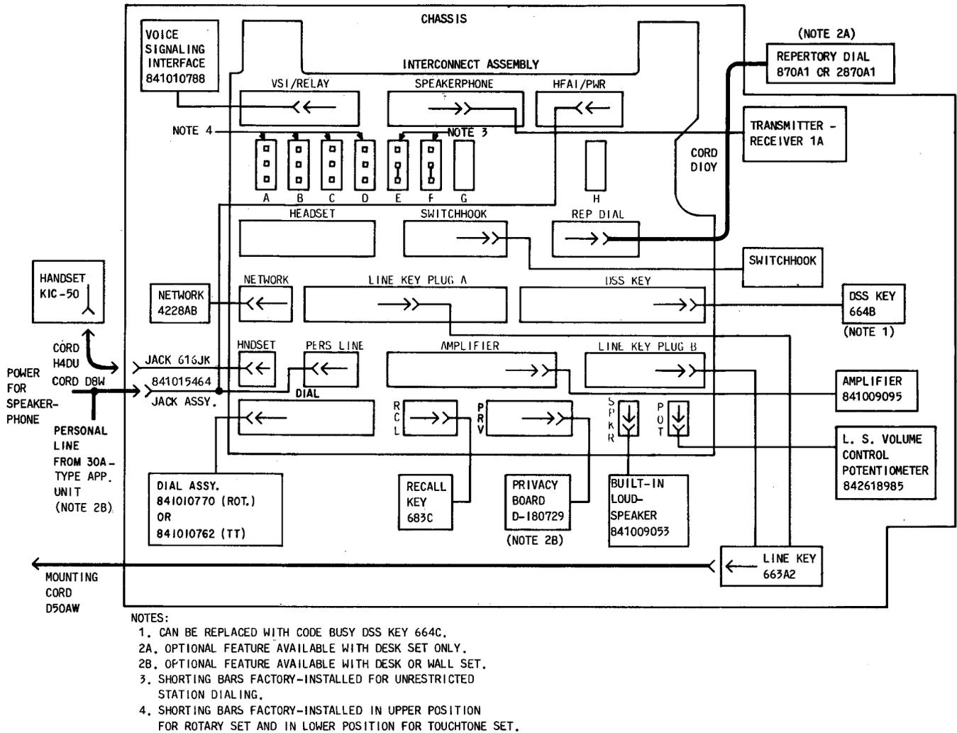
Fig. 51—Block Diagram of BIS Satellite Set
