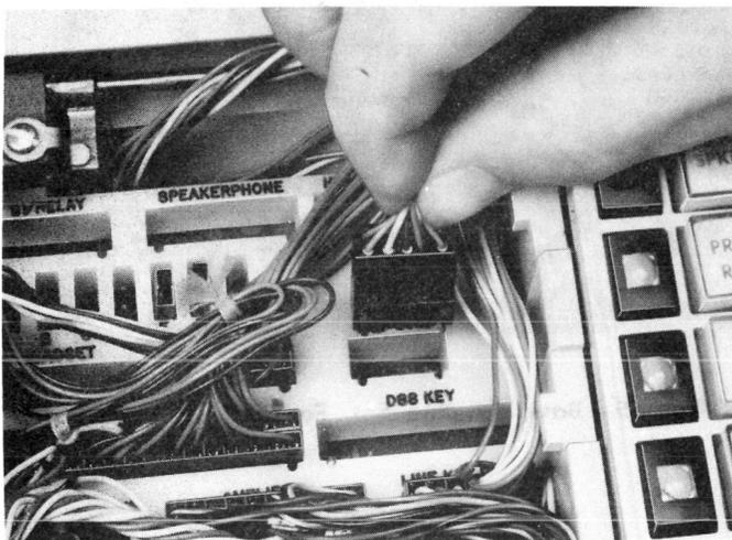
Fig. 57—Unplugging a Component Connector From Interconnect Field
