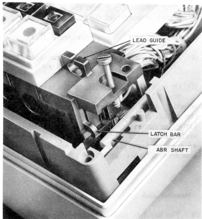
**Fig. 58—Line Key Installation**
