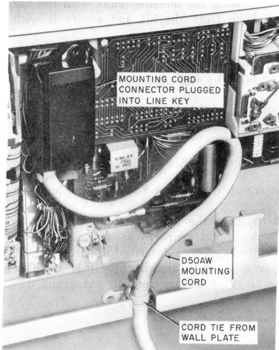
**Fig. 17—D50AW Mounting Cord Connected to Wall Set**
