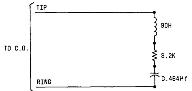
Fig. 2—1A Termination Unit, Connections
