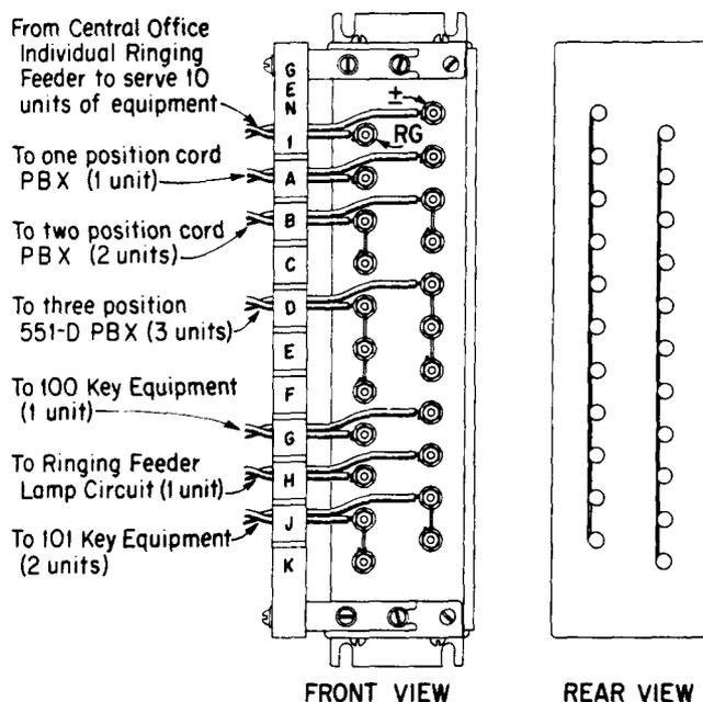
Fig. 1—Typical Arrangement Showing the Termination and Strapping of Ringing Leads at a Centralized Ringing Feeder Panel on Customer's Premises
