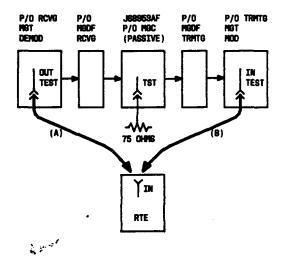
NOTE: 86 PILOT LEVEL AT OUT TEST AND IN TEST JACKS IS APPROXIMATELY -80.0 DBM
