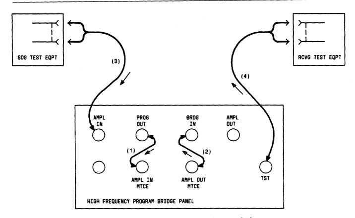
Fig. 4—Patching at High Frequency Program Bridge
