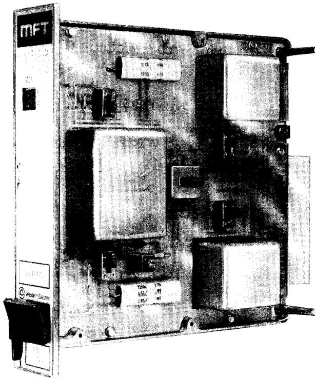
Fig. 5—Two-Wire Transmission Unit J99343BC
