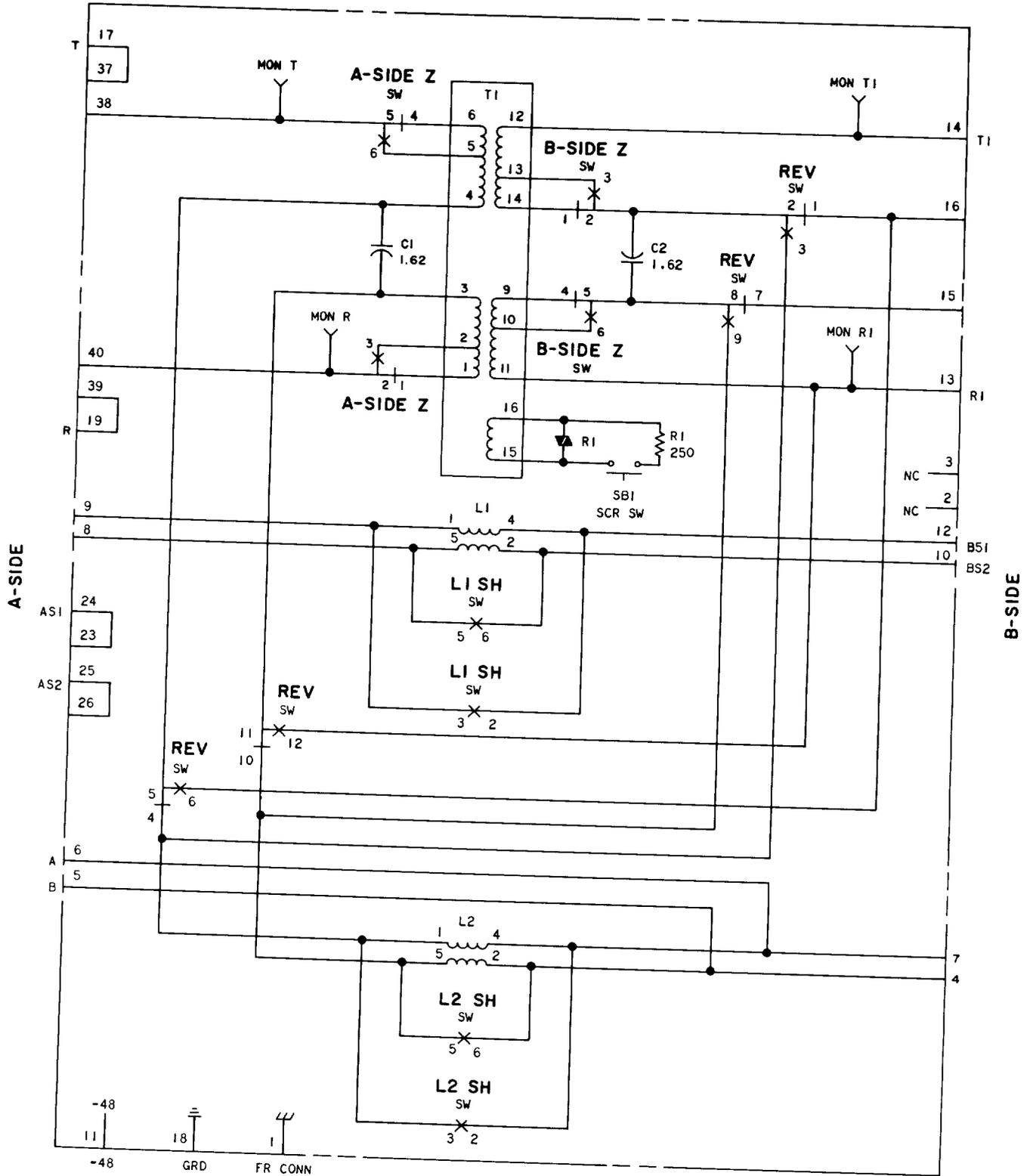
Fig. 6—Schematic of J99343BC 2-Wire Transmission Unit
