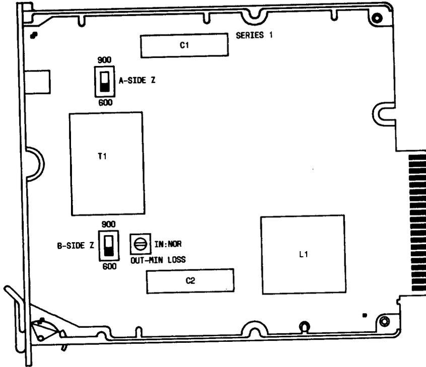
◆ Fig. 7—ATP-4 600/900 dc Bypass Unit ◆
