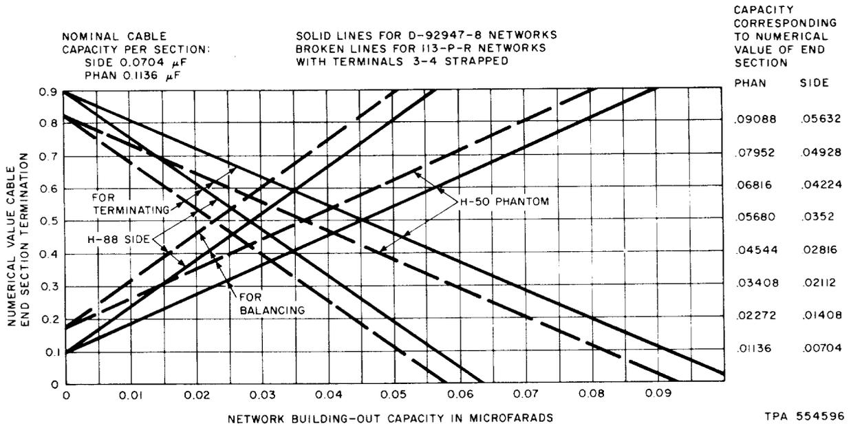
Fig. 8—Network Building-Out Capacity vs Cable End-Section for H-88-50 Balancing Networks
