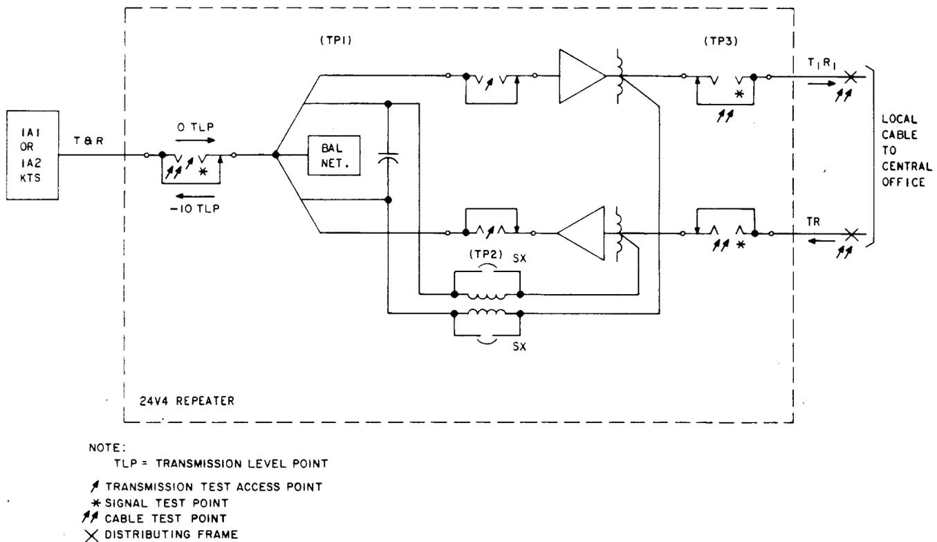
Fig. 1—Typical 2-Wire Station Termination Test Access Points
