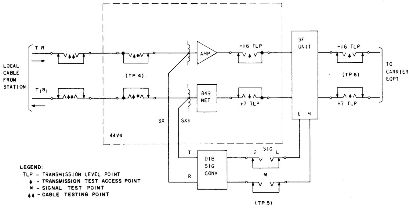
Fig. 3—Typical Central Office Arrangement for Two-Point Private Line Telephone Service and Test Access Points
