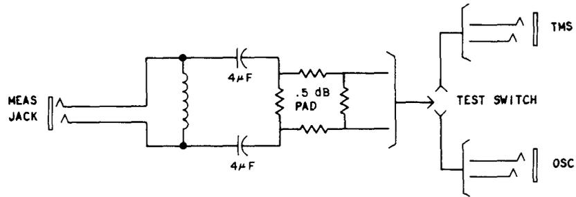
FIG. 4A 2AB SET USED FOR DC ISOLATION
