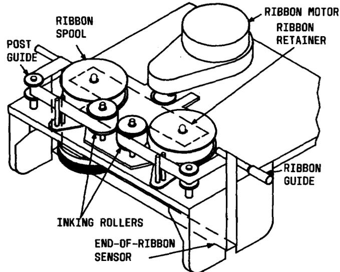
Fig. 8—Replacing Ribbon
