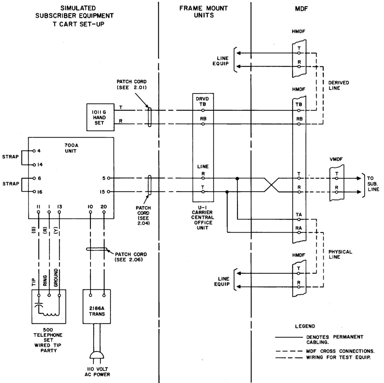
Fig. 1—Central Office U1 Carrier Test Arrangement
