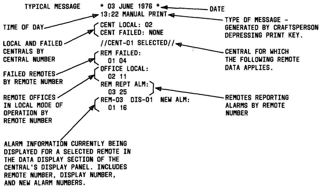
Fig. 4—Typical Printer Message for Central
