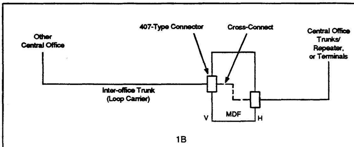
Figure 1. Typical Application with Digital Loop Carrier Systems (Sheet 2 of 2)
