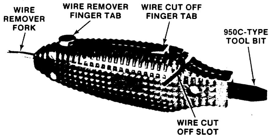
Figure 3. 950C-Type Wire Insertion/Removal/Cutter Tool
