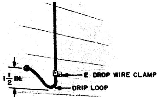
Fig. 2 - E Drop Wire Clamp Installed
