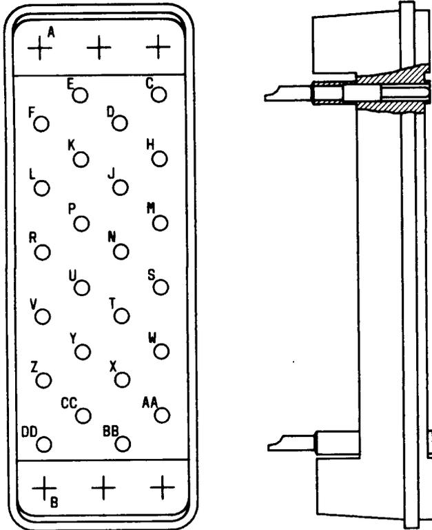
Fig. 3—KS-20669, L1 Through L21, Connectors
