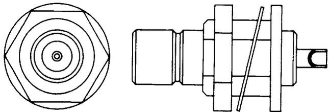
Fig. 12—KS-20863, L4, L5, L6, or L13, Connector
