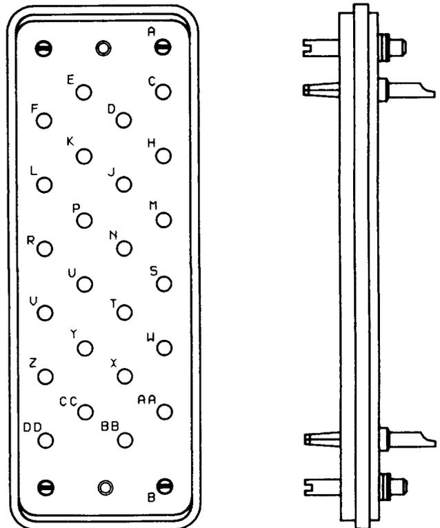
Fig. 2—KS-20668, L1 Through L16, Connectors
