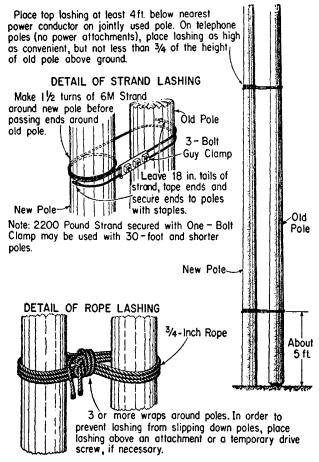
3.03 In order to place the upper lashing, climb the new pole. Do not, under any circumstances, work from the old pole until both upper and lower lashings have been completed. Rope lashings should be used only where the old pole is to be removed within a reasonable period of time (usually a few days) or where there might otherwise be an electrical hazard in passing the sling around the poles.
