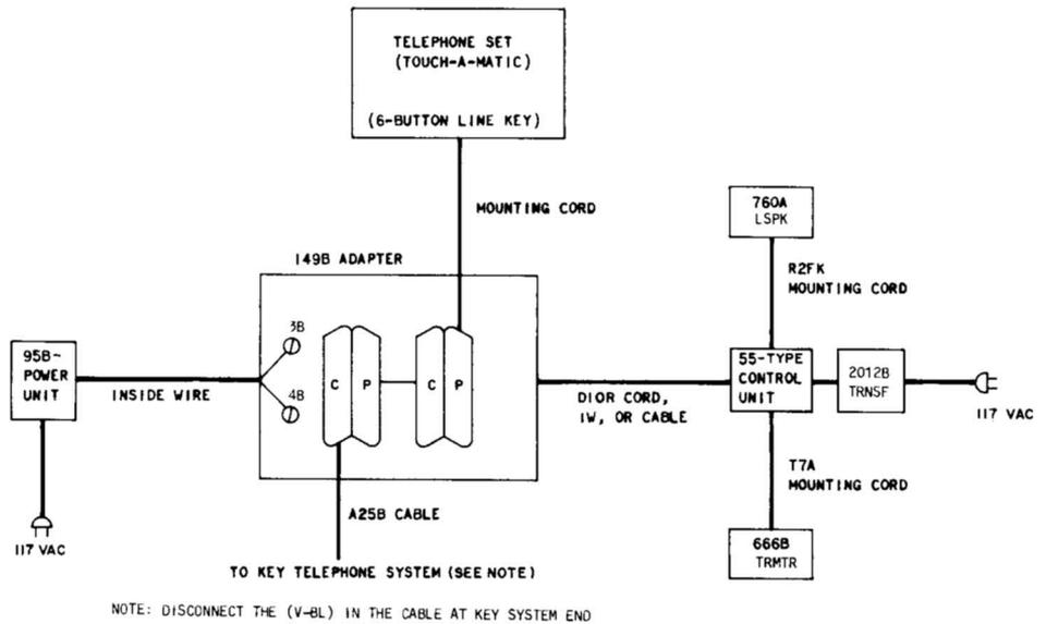
Fig. 10—Block Diagram—872A1M Telephone Set Using 3B Speakerphone
