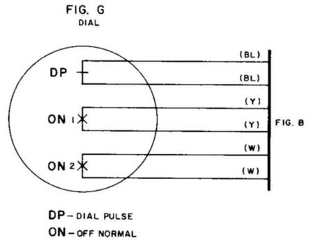
Fig. 8—872A1M Telephone Set, Connections (Sheet 2 of 4)
