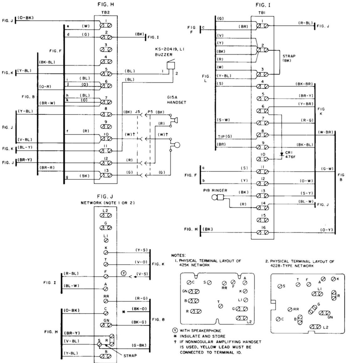
Fig. 8—872A1M Telephone Set, Connections (Sheet 3 of 4)
