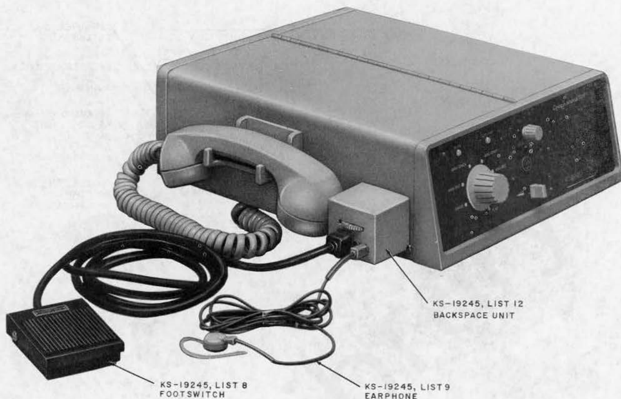
Fig. 24—KS-19245, List 1 Telephone Answering Set—With Accessories
