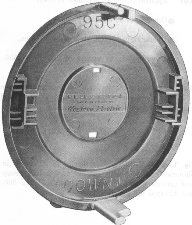
Fig. 4—95C (Current Model) —Similar in frontal appearance to the 95C (early model). Equipped with ribs which provide frictional fit to dial mounting bracket on sets having 2 and 3 point suspension.
