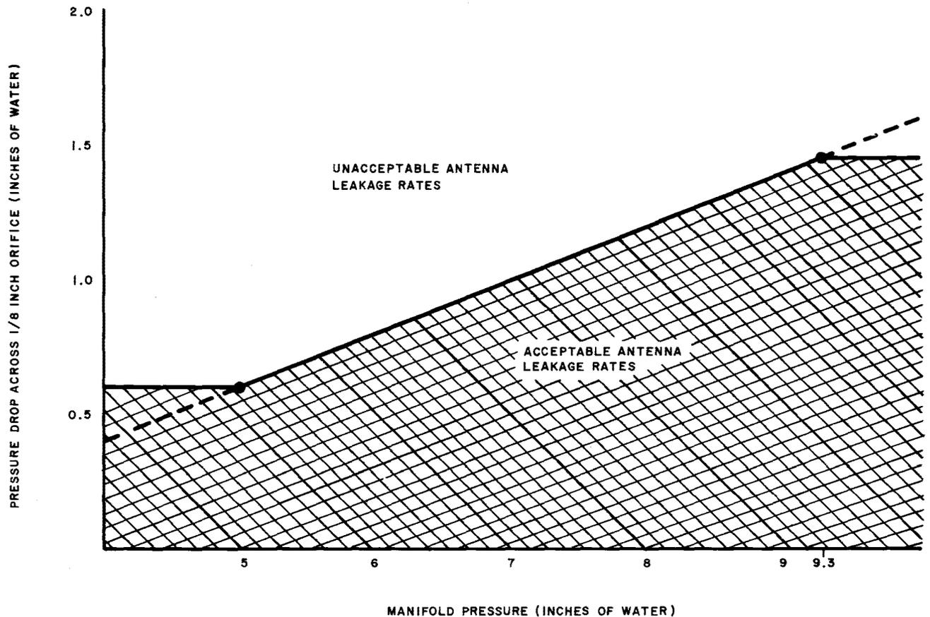
Fig. 3—Air Leakage Chart
