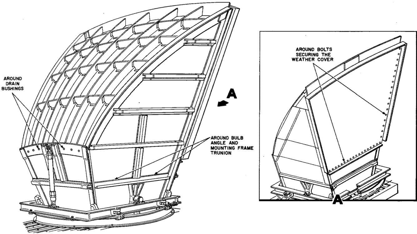
Fig. 6—Common Source of Seal Leakage
