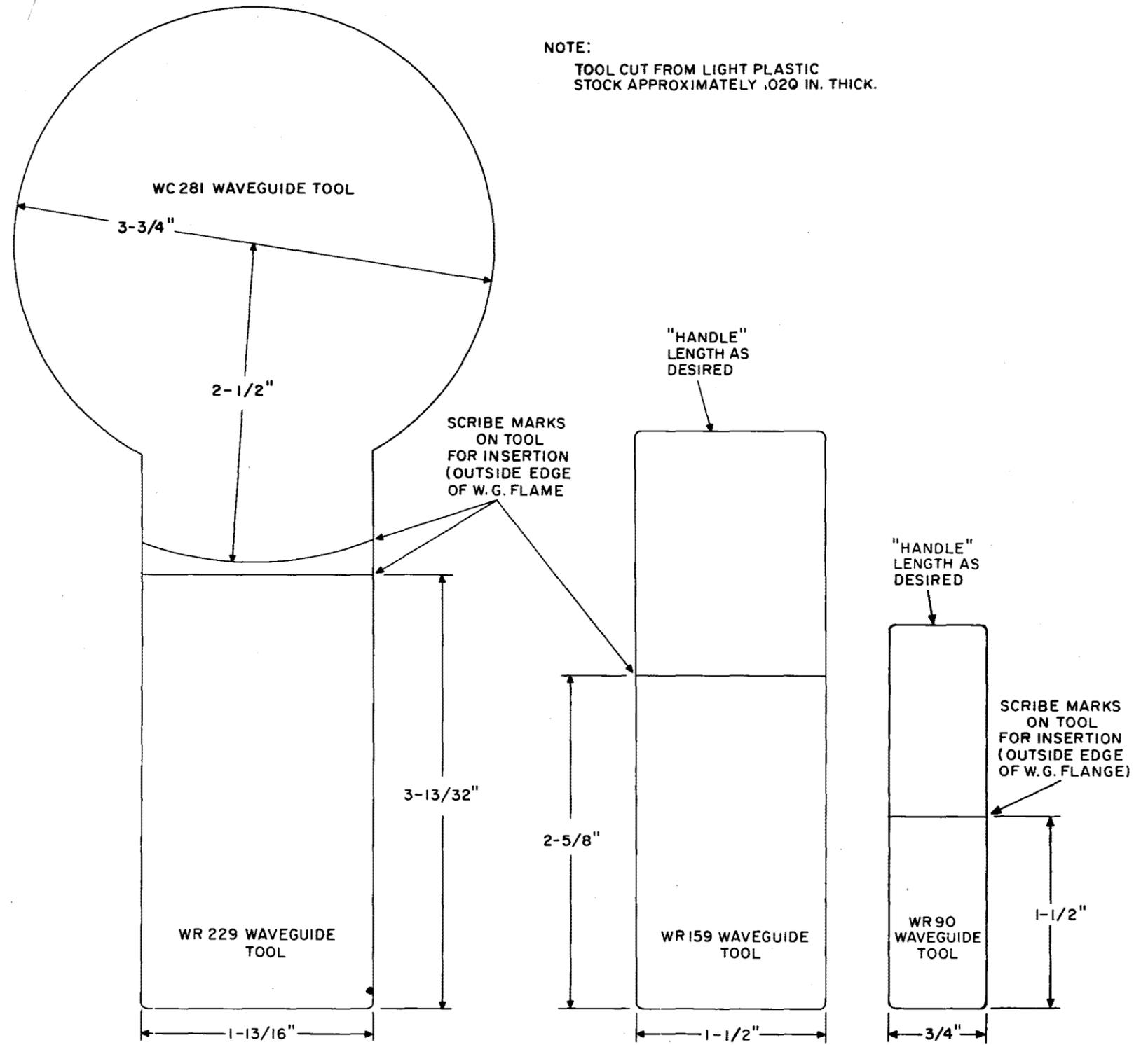
Fig. 4—Template for Air Blocking Tool
