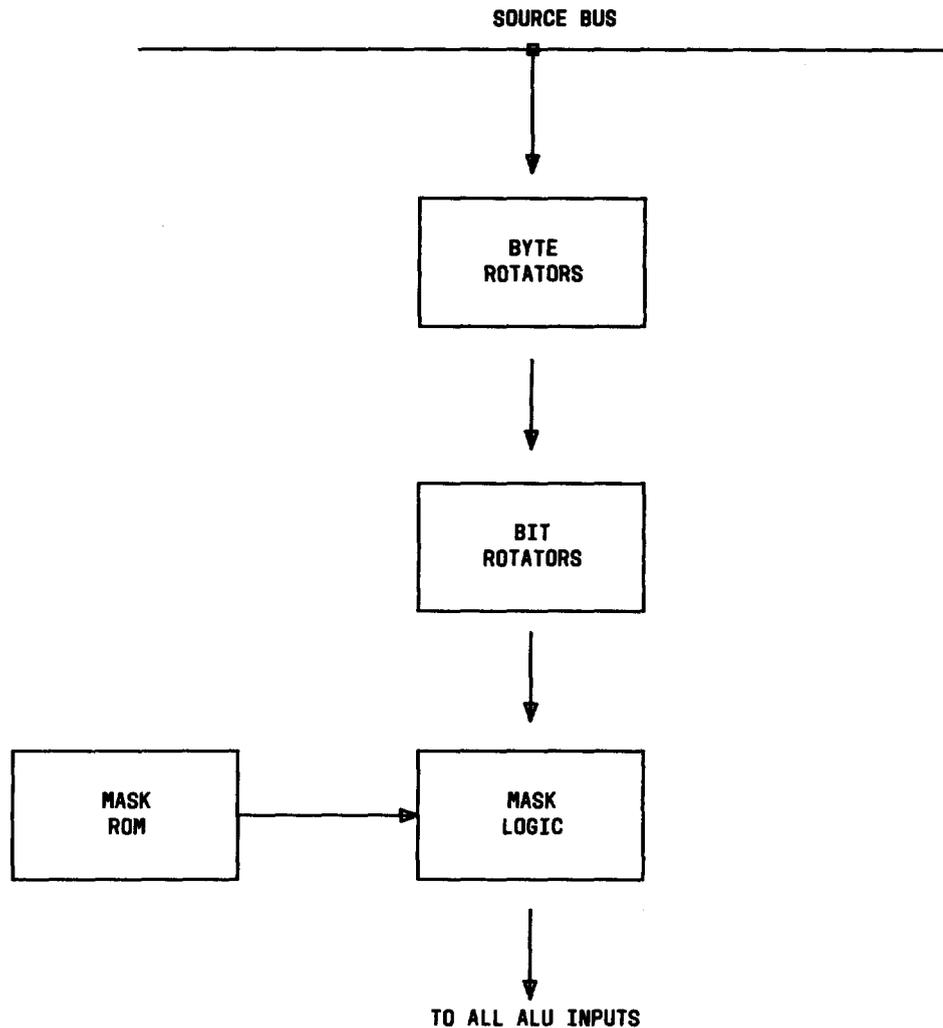
Fig. 11—Rotate Mask Unit
