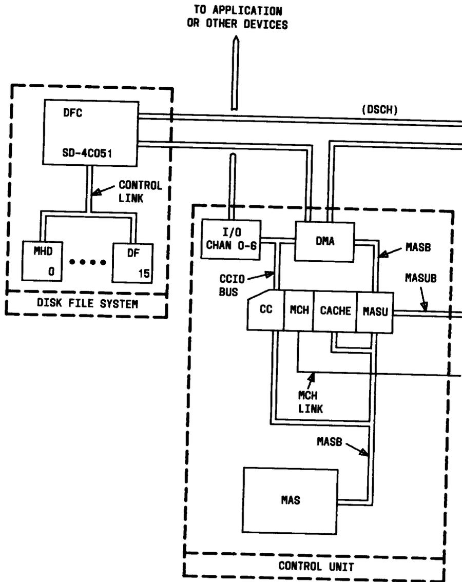
Fig. 5—3B 20D Model 1 Computer—Functional Overview (Sheet 1 of 2)
