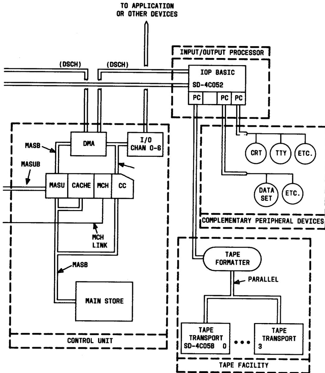
Fig. 5—3B 2D Model 1 Computer—Functional Overview (Sheet 2 of 2)
