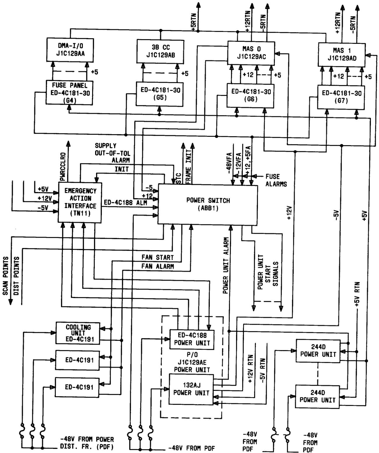
Fig. 34—Control Unit Frame Power Distribution, Control, and Alarms
