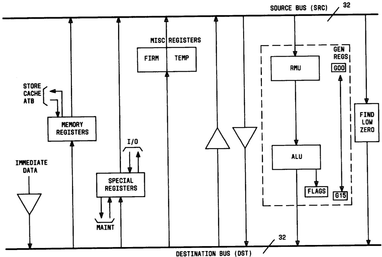
Fig. 6—Internal CC Architecture Block Diagram
