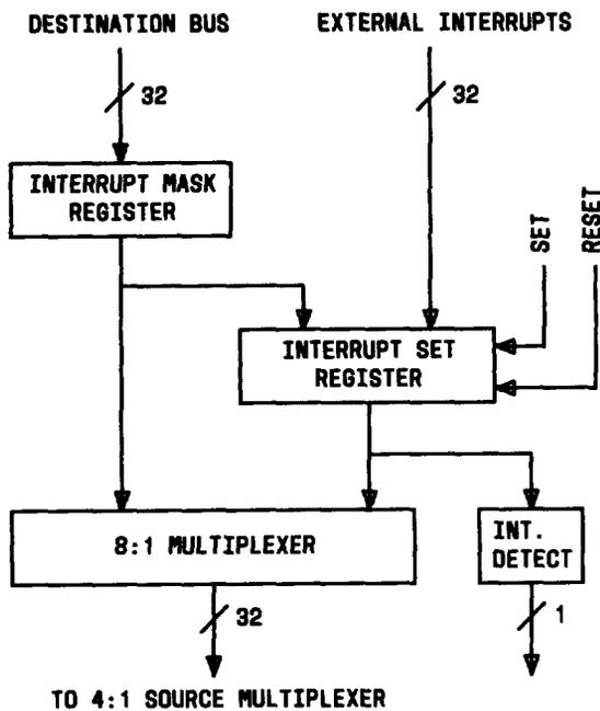
Fig. 25—Interrupt Set and Interrupt Mask Registers
