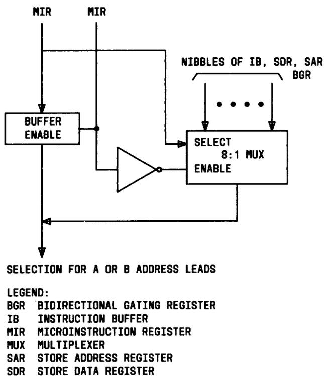
Fig. 14—A and B Address Control
