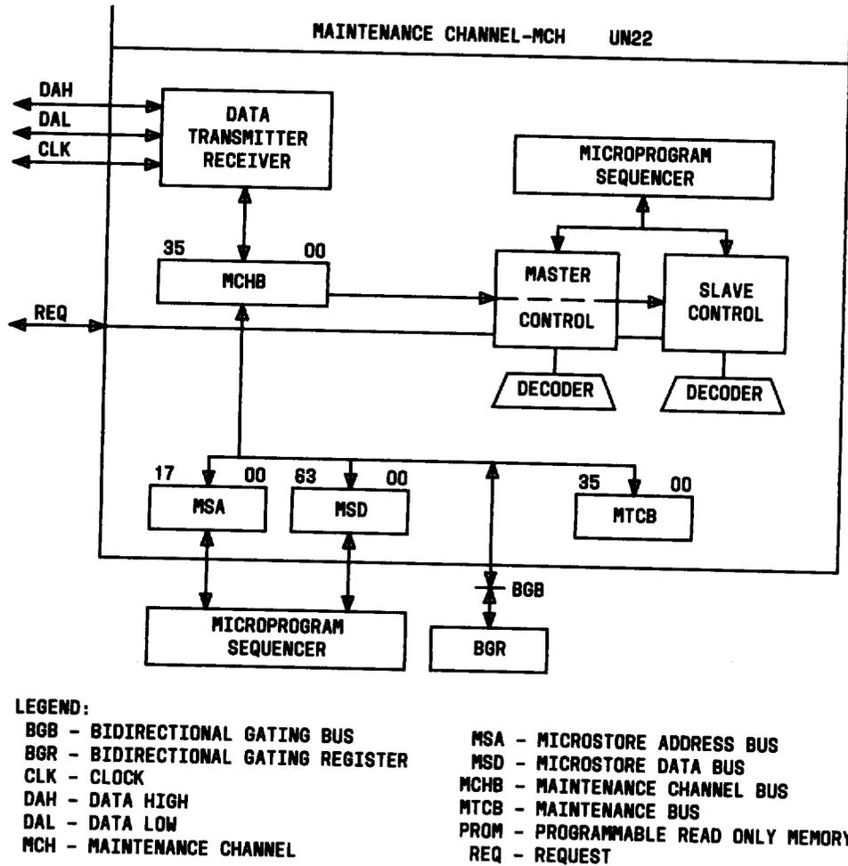
Fig. 27—Maintenance Channel Block Diagram
