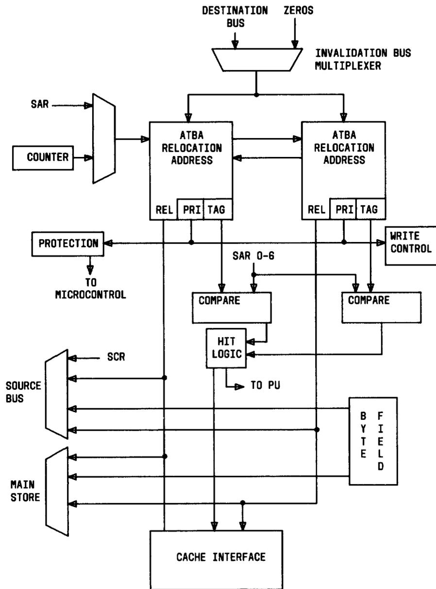
Fig. 18—Store Address Translator Block Diagram
