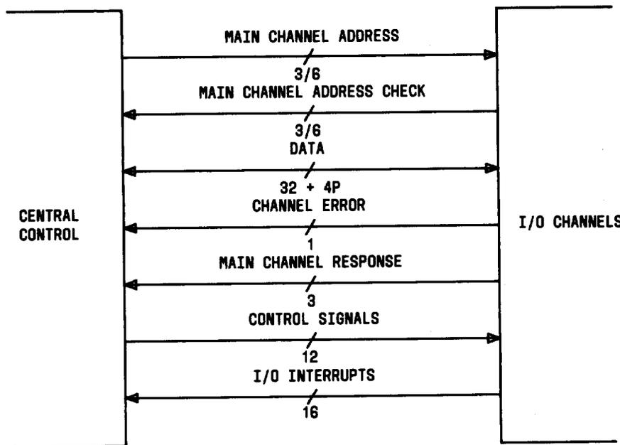
Fig. 4—3B 20D Model 1 Computer CCIO Bus
