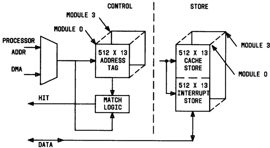
Fig. 28—Cache Store Unit Block Diagram
