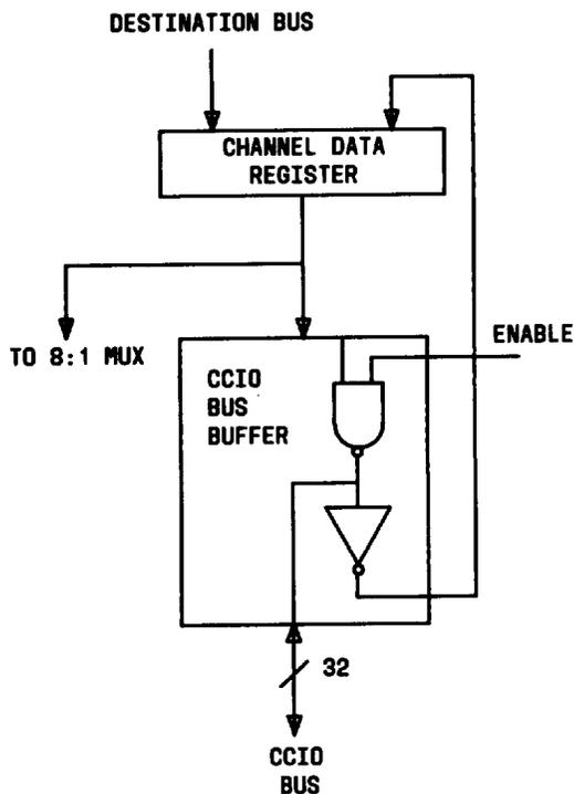
Fig. 17—Channel Data Register Diagram
