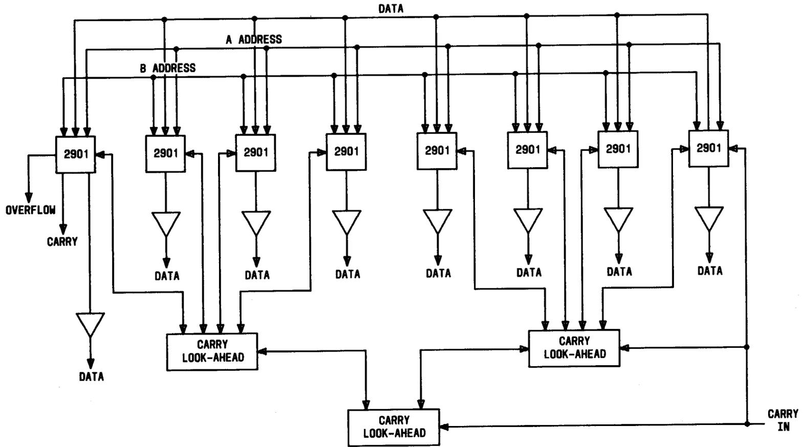
Fig. 15—Arithmetic Logic Unit, Internal Architecture
