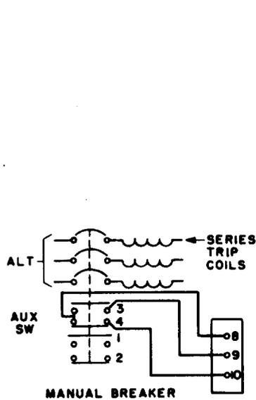
**Fig. 6 – KS-15910, L3 and L4 Schematic**
