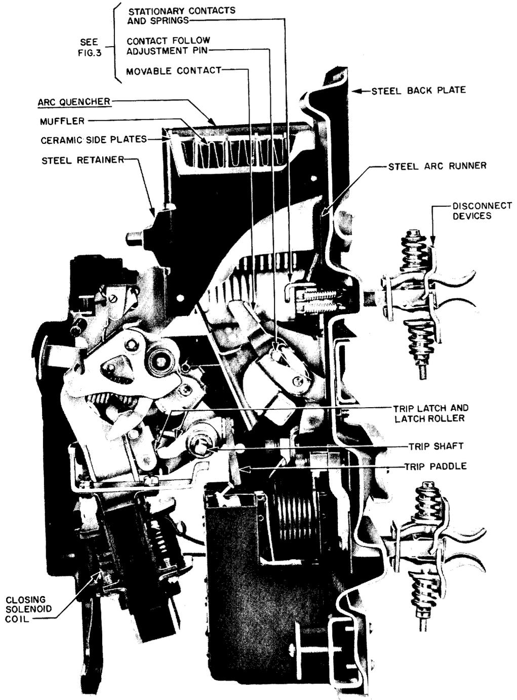
Fig. 2 - Cut-Away View of Electrically Operated Breakers - Reset Position
