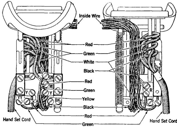
Fig. 5-214A Type Hand Telephone Sets.
