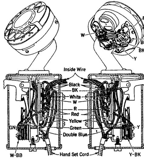
Fig. 6-201B, 201C, 201D Type Hand Telephone Sets.
