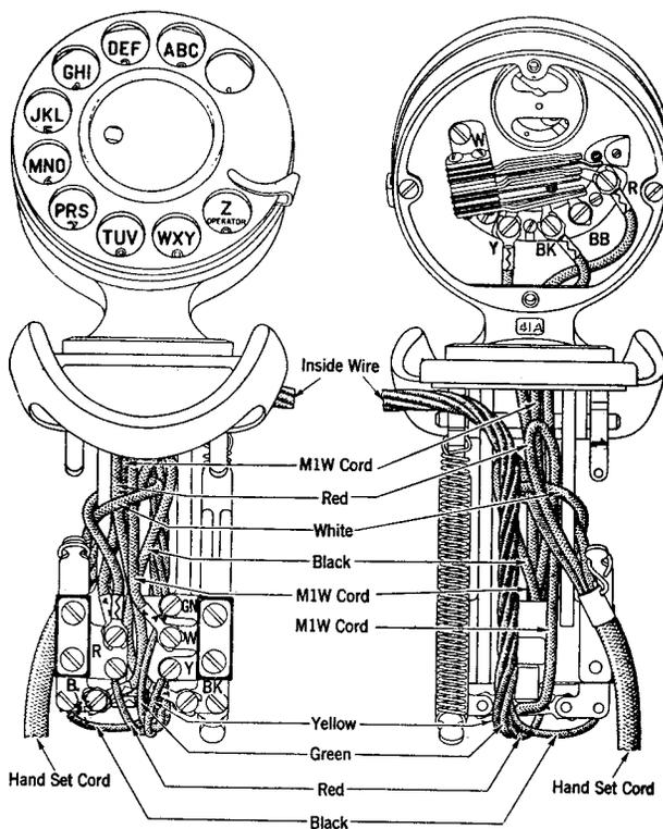
Fig. 8—211F, 211G, 211H Type Hand Telephone Sets.
