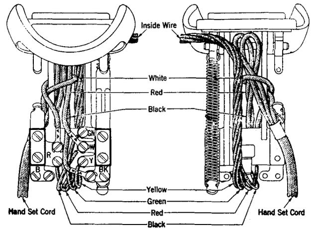
Fig. 3—211E Type Hand Telephone Sets.
