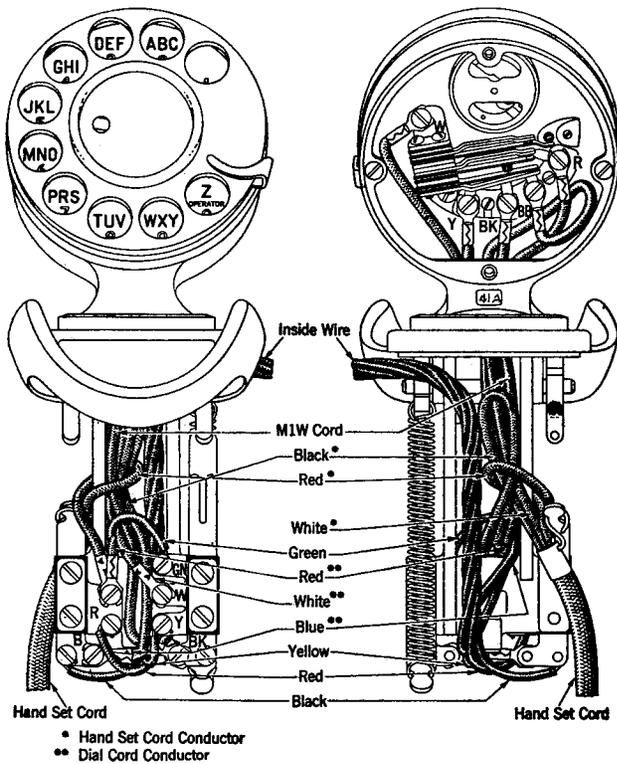
Fig. 7—211B, 211C, 211D Type Hand Telephone Sets.
