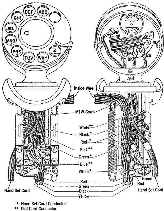
Fig. 11—214B, 214C, 214D Type Hand Telephone Sets.
