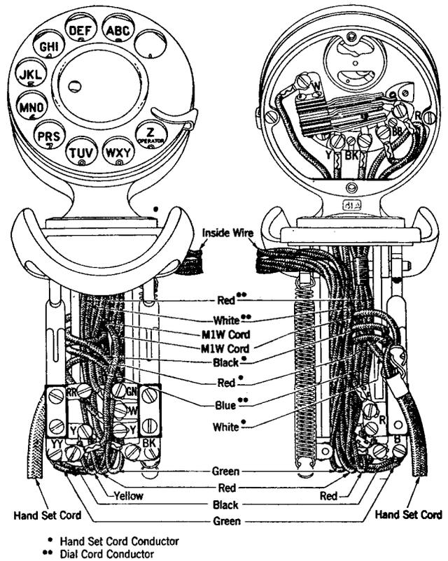
Fig. 9—212A, 212B, 212C Type Hand Telephone Sets.
