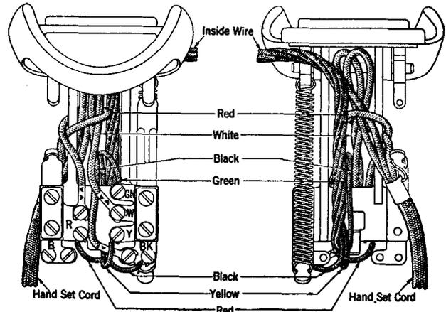
Fig. 2—211A Type Hand Telephone Sets.
