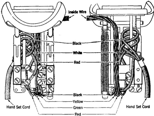
Fig. 4-213E Type Hand Telephone Sets.
