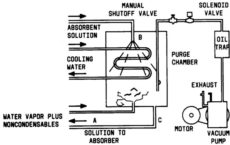
Fig. 13—Schematic of Purge System
