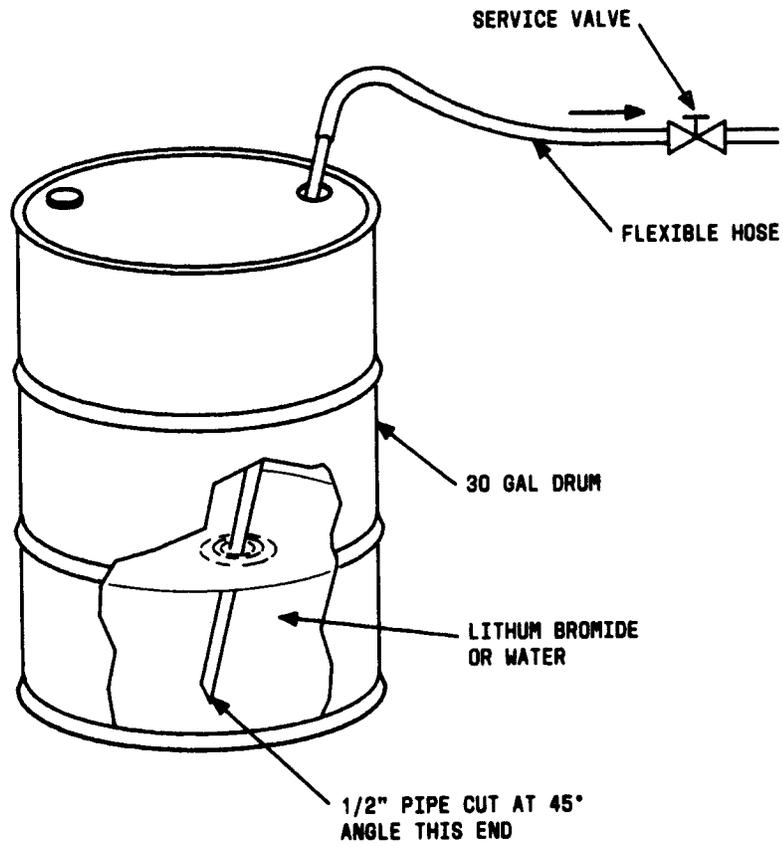
Fig. 18—Charging Solution and Refrigerant
