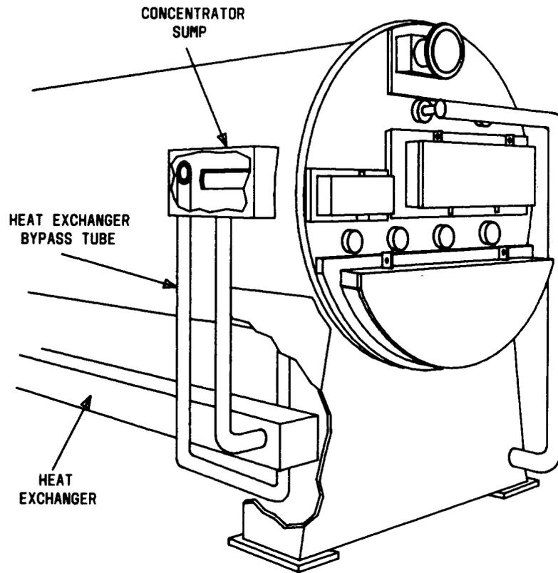
Fig. 8—Heat Exchanger Bypass
