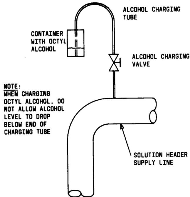
Fig. 14—Alcohol Charging Connection
