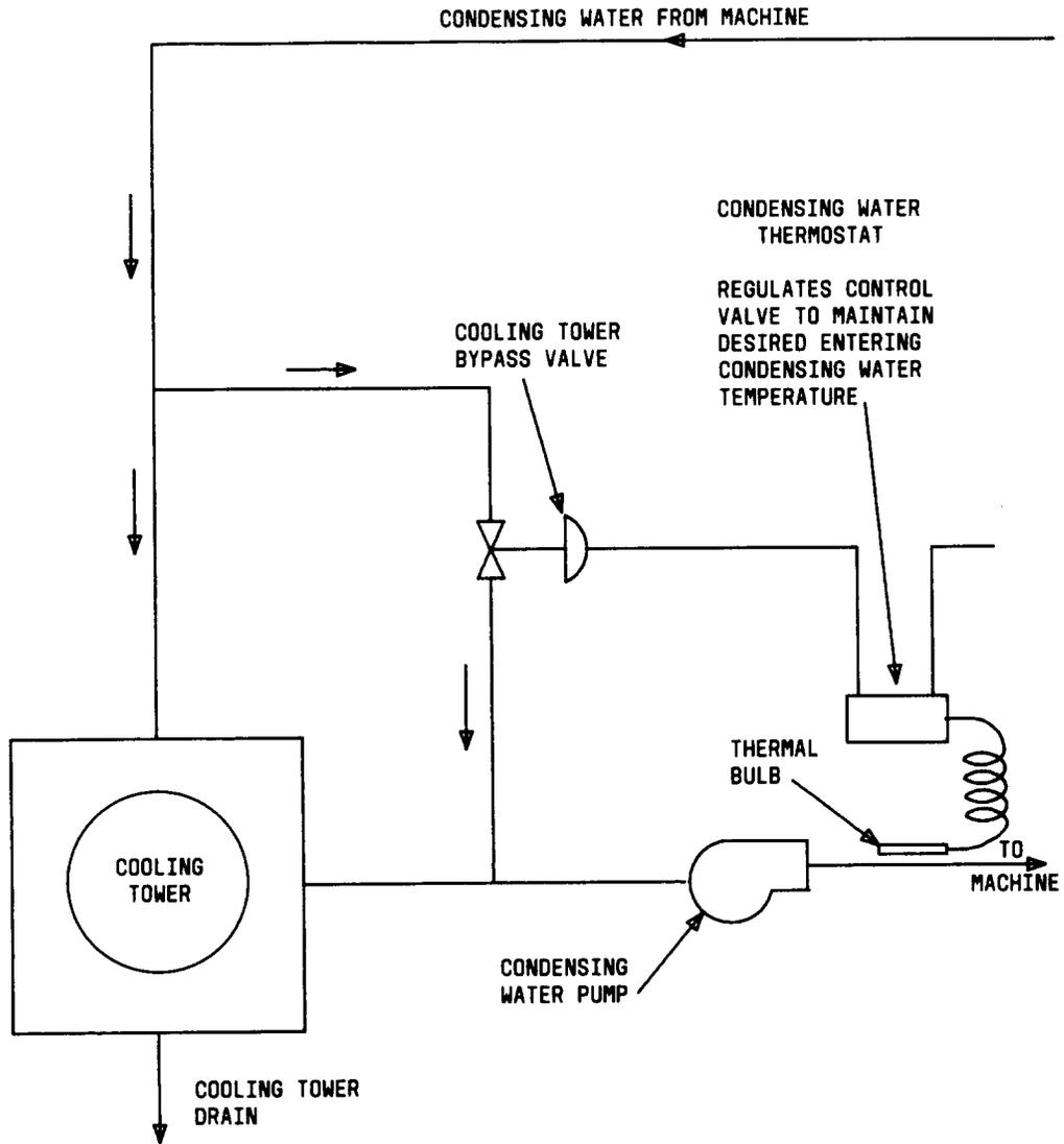
Fig. 9—Cooling Tower Circuit
