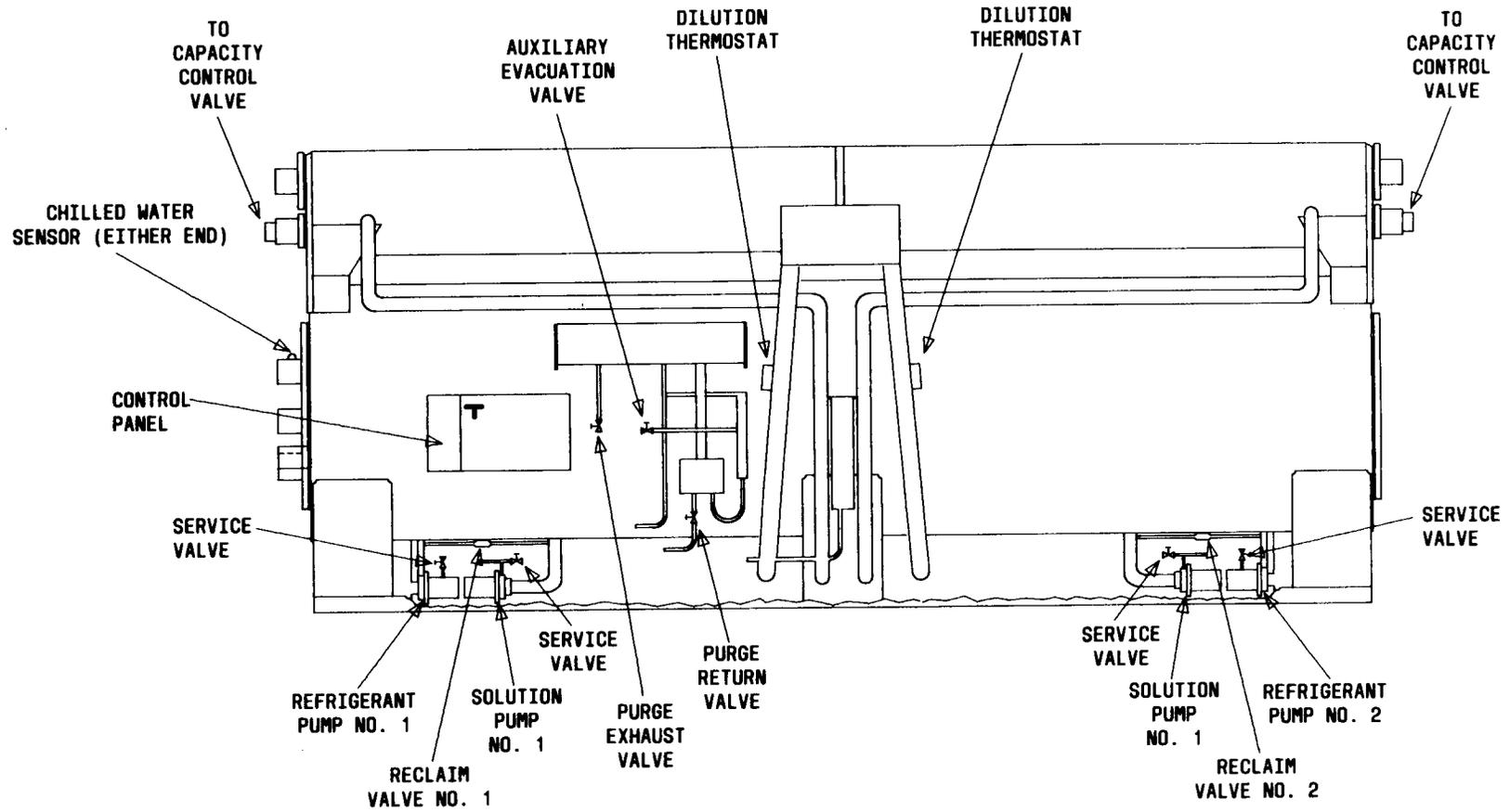
Fig. 16—Solution or Refrigerant Sampling
