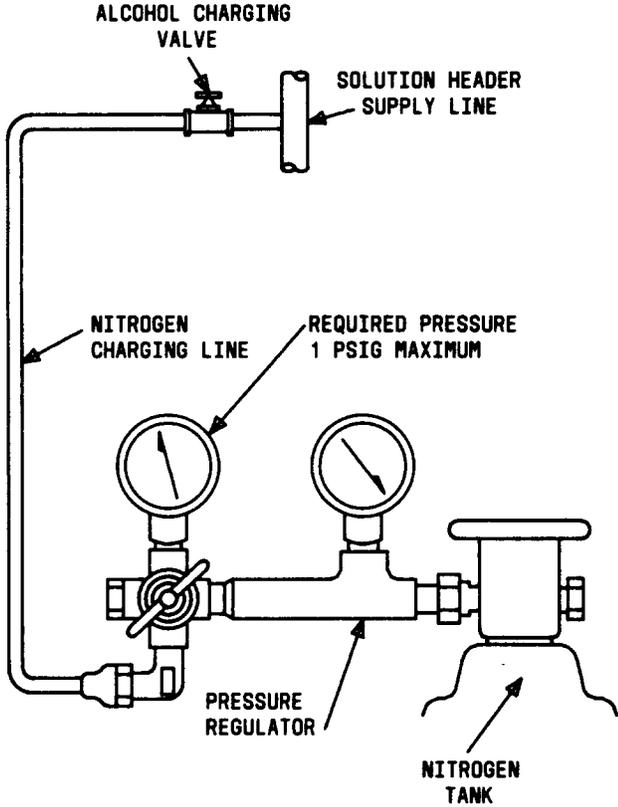
Fig. 19—Nitrogen Manifold
