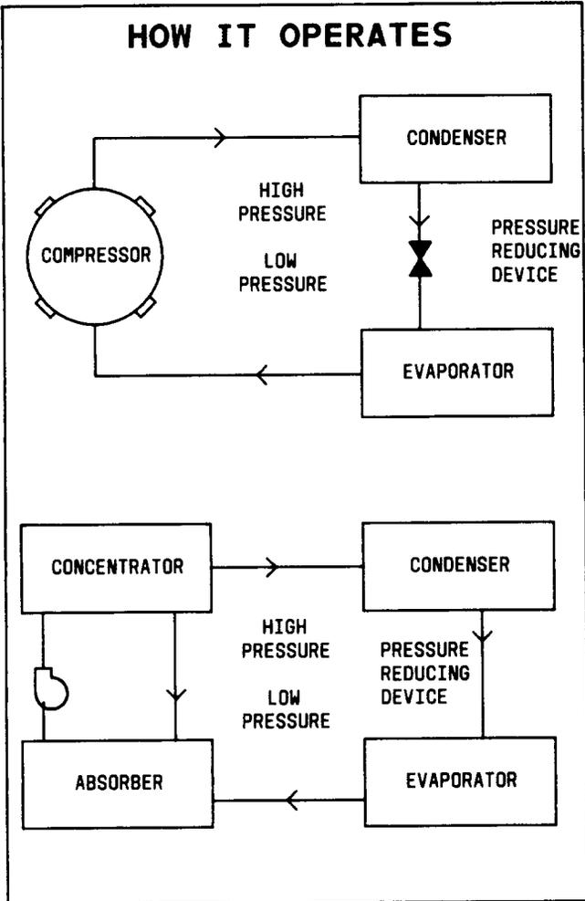
Fig. 2—Comparison of Mechanical Refrigeration Cycle and Absorption Refrigeration Cycle
