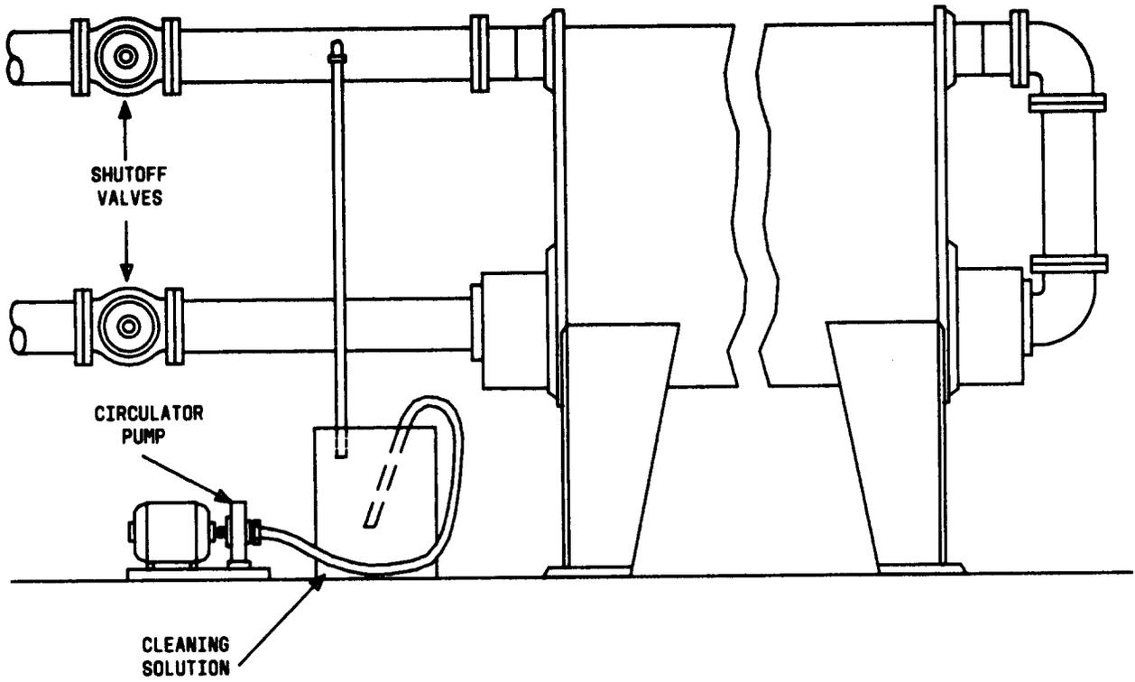
Fig. 15—Typical Tube Cleaning Hookup
