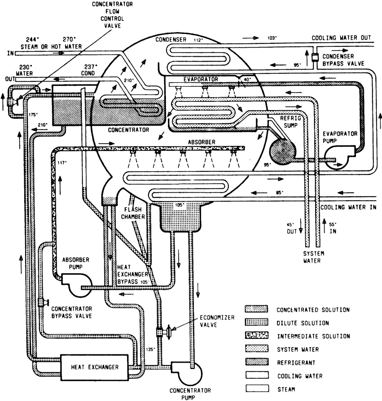
Fig. 4—Schematic of Absorption Cycle
