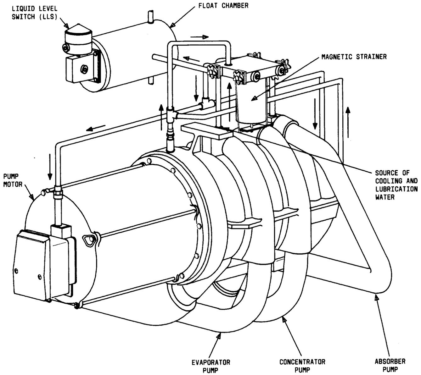
Fig. 7—Pump Motor Lubricating and Cooling Circuit
