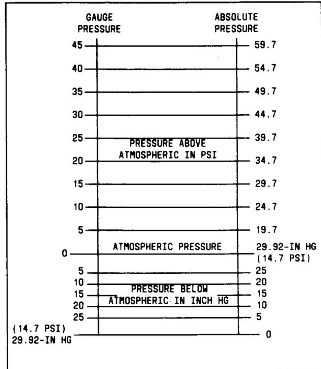
Fig. 3—Relationship Between Absolute and Gauge Pressures
