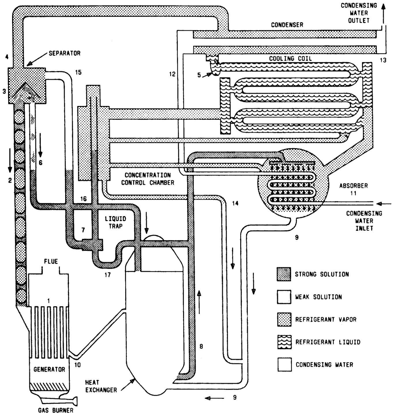
Fig. 6—Cooling Cycle—Schematic Flow Diagram—Single Coil, Direct Fired Unit
