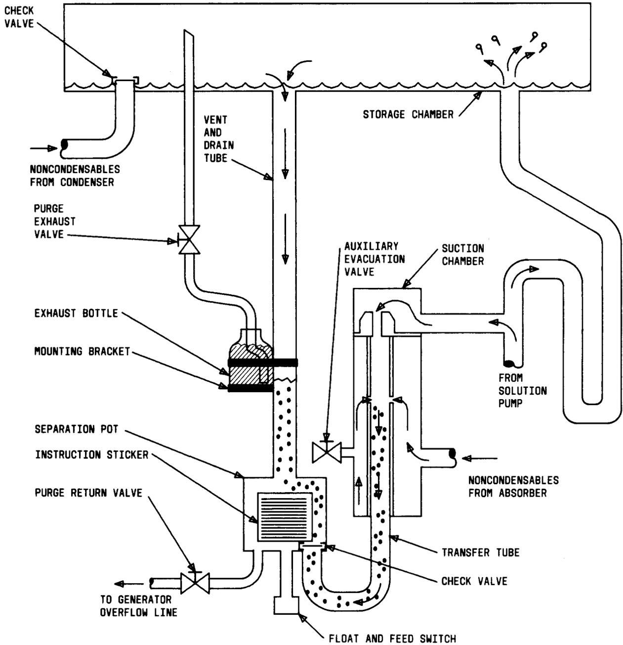
Fig. 12—Typical Nonmechanical Purge Unit
