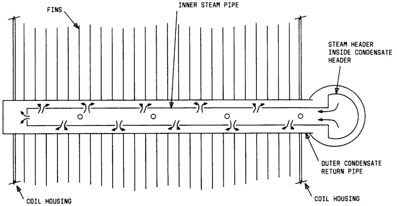
Fig. 2—Nonfreeze or Double Tube Steam Coil
