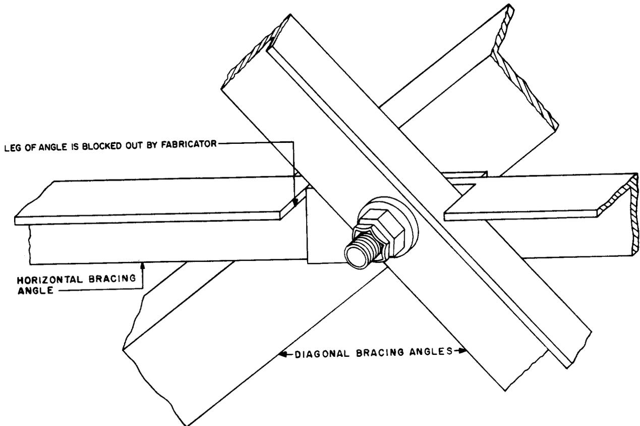
Fig. 7 - Diagonal and Horizontal Bracing Crossover Connection
