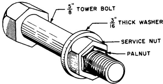
Fig. 5 - Tower Bolt Assembly
