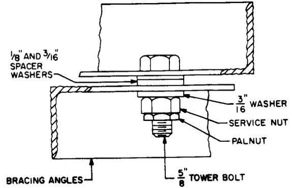
Fig. 6 - Diagonal Bracing Crossover Using Spacer Washers
