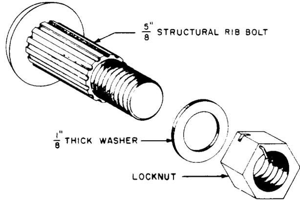
Fig. 3 - Structural Rib Bolt Assembly
