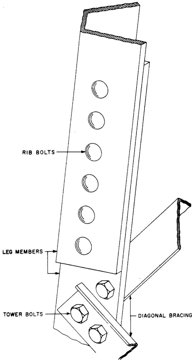
Fig. 2 - Lap Splice and Bracing Connections
