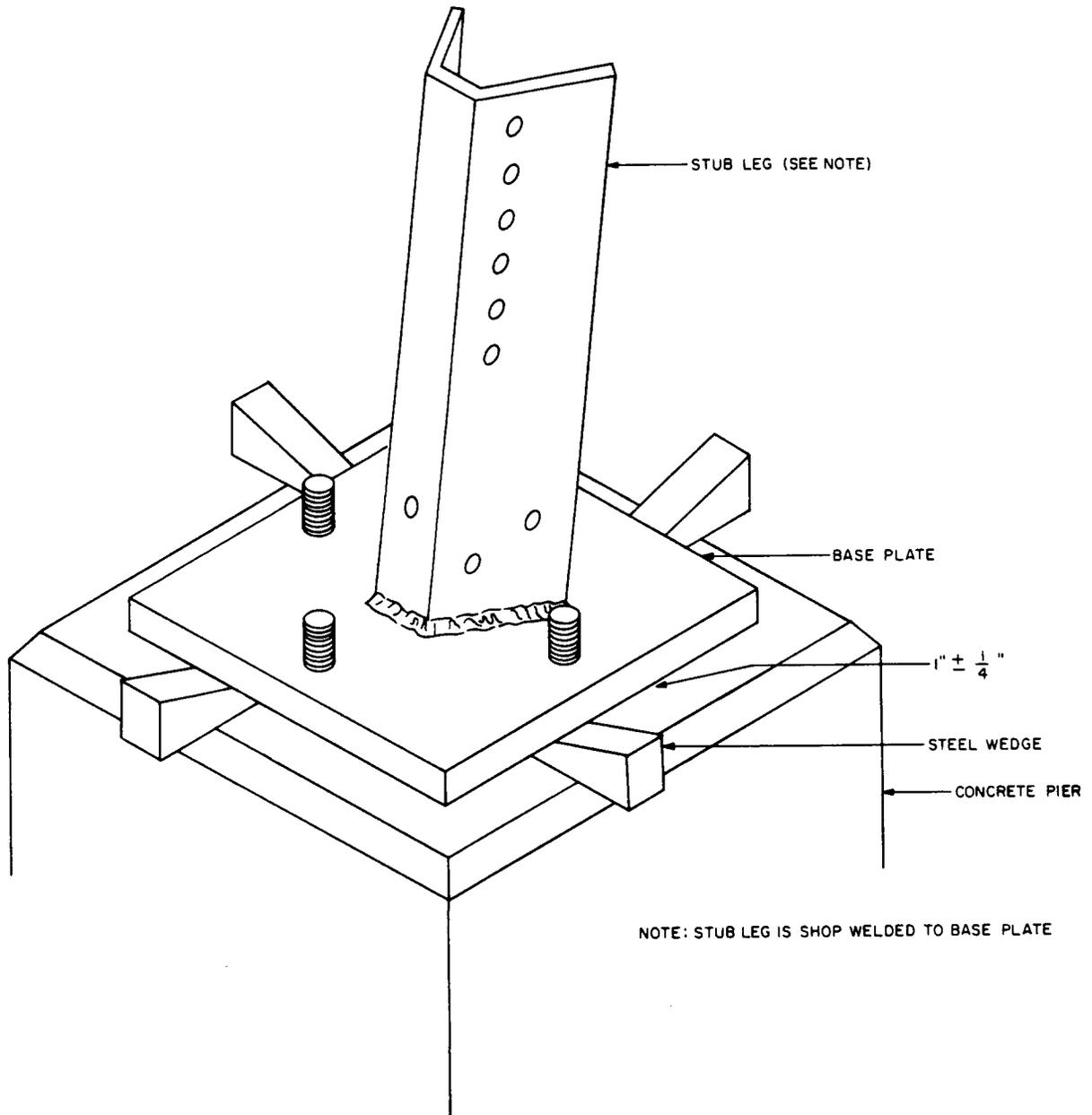
Fig. 1 - Installation of Base Plate Assembly
