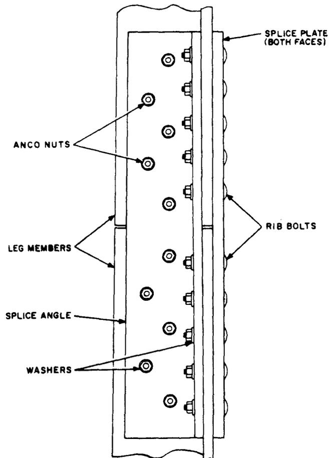
Fig. 8—Butt Leg Splice
