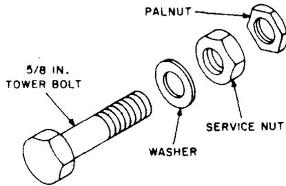
**Fig. 4—Typical Bolt Assembly**
