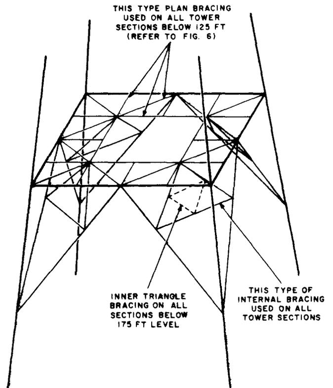
**Fig. 7—Tower Bracing**
