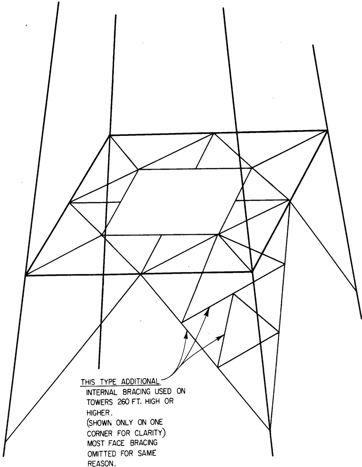
Fig. 6 - Types of Internal Bracing
