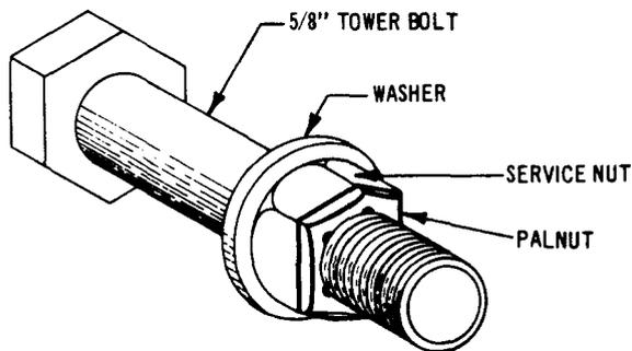
Fig. 4 – Typical Bolt Assembly
