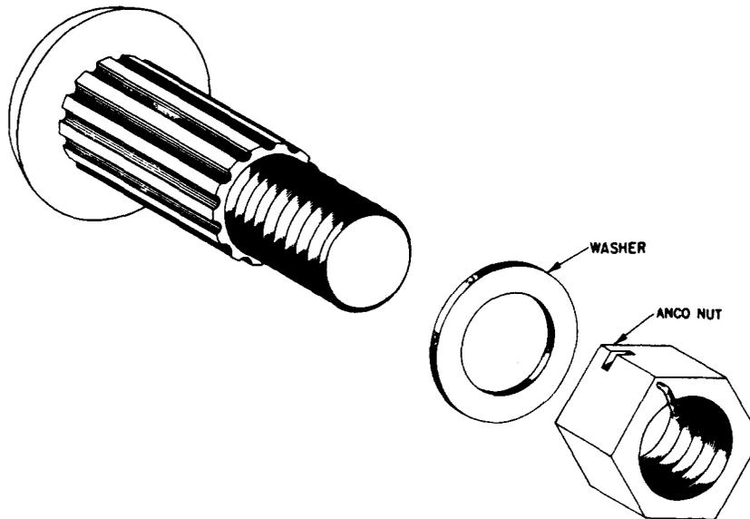
Fig. 2 – Structural Rib Bolt Assembly
