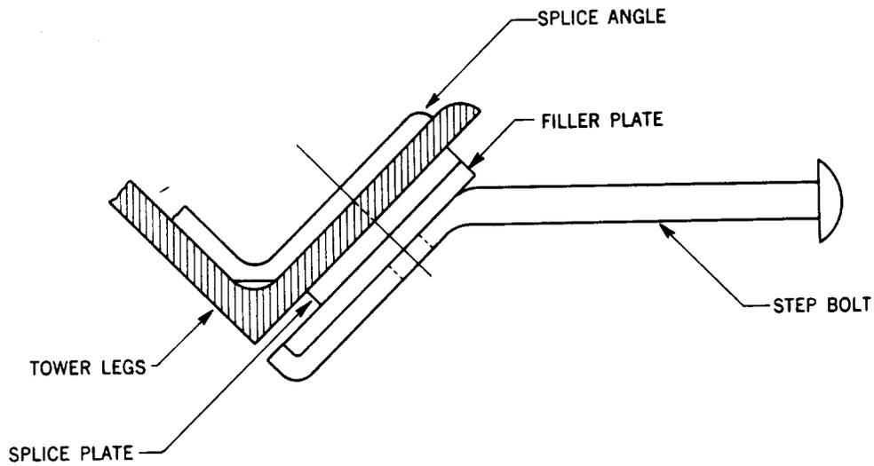
Fig. 13 - Typical Step Bolt at Leg Splice
