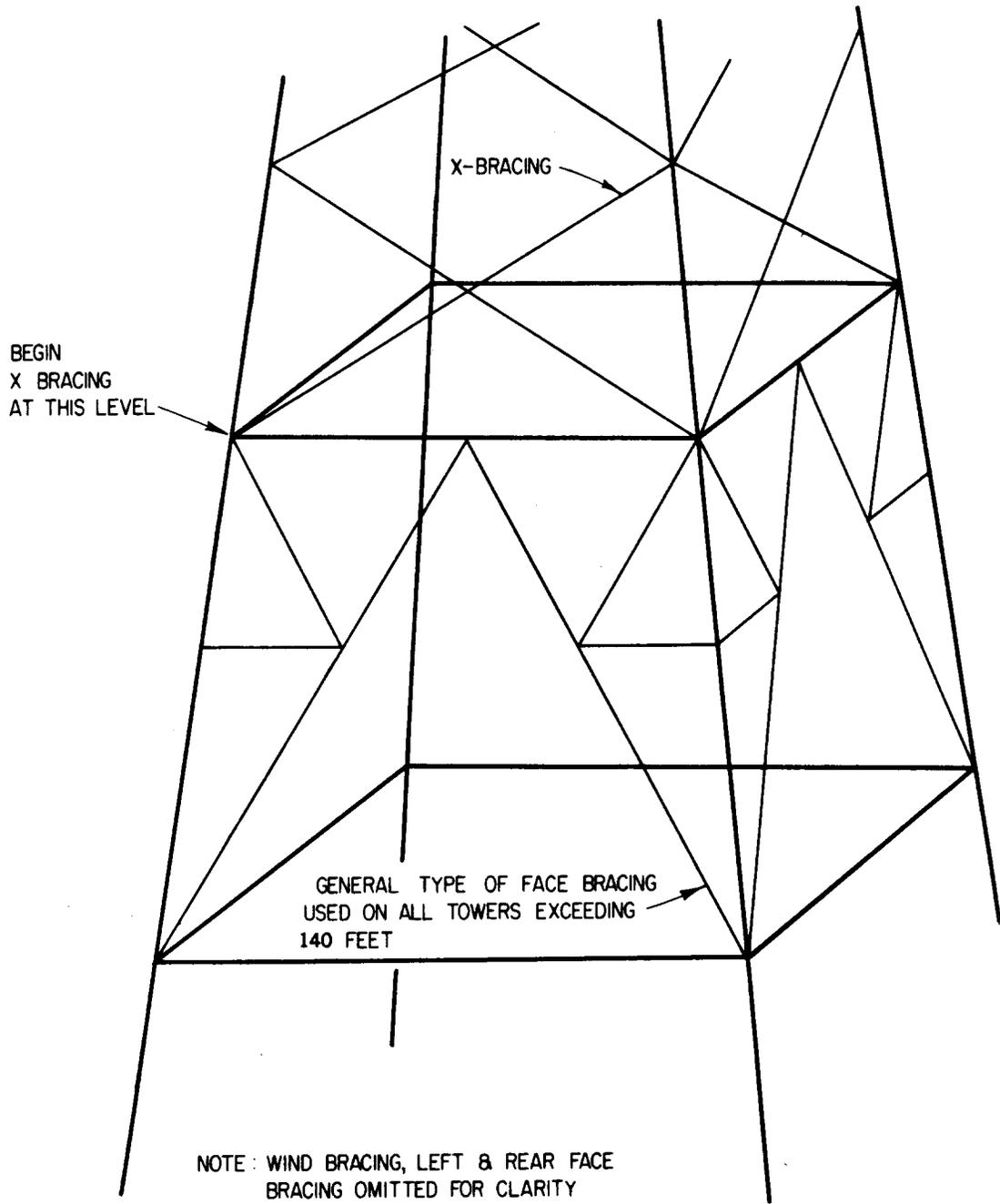
Fig. 10 - Types of Face Bracing
