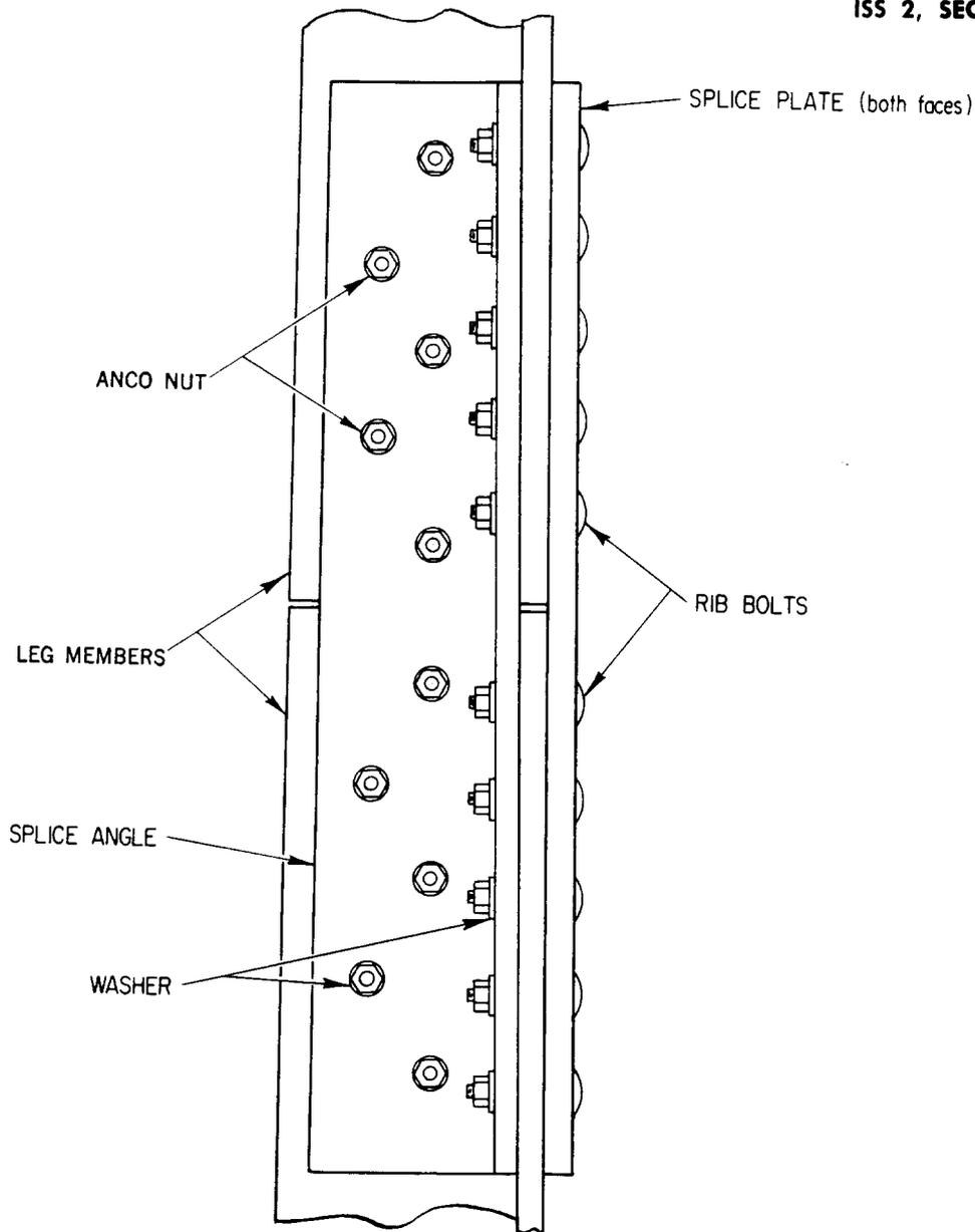
Fig. 7 - Typical Butt Splice
