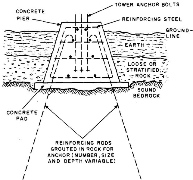
Fig. 1—Typical Foundation in Rock
