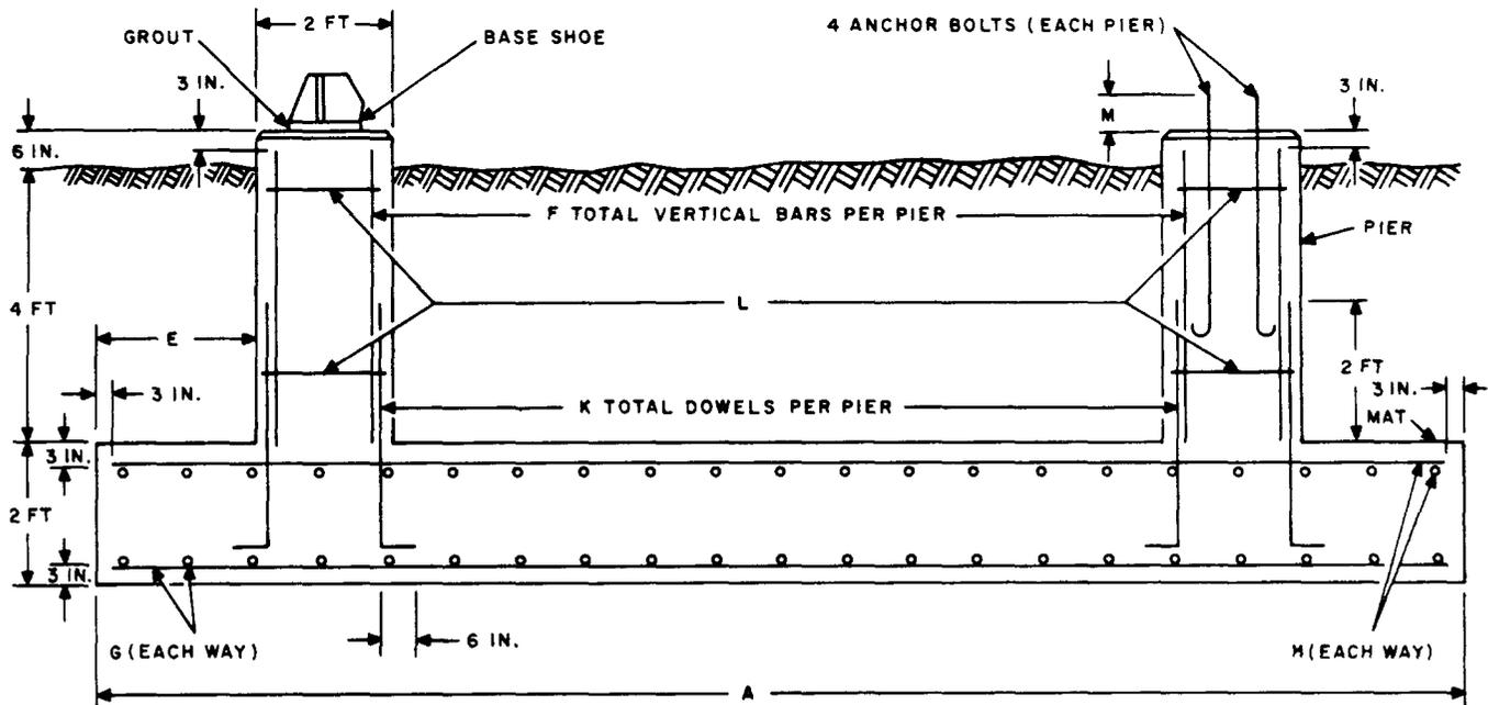
Fig. 2—Cross-Sectional View—Foundations for Towers From 40 Through 100 Feet in Height
