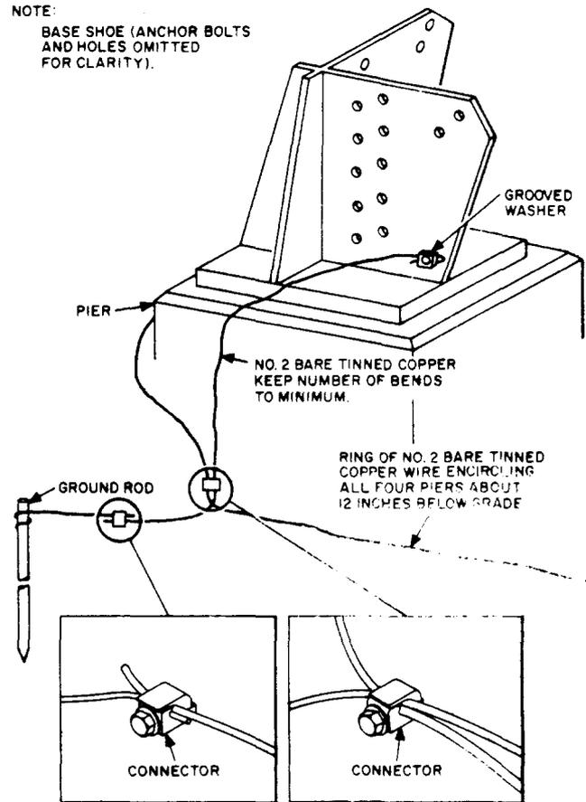
Fig. 8—Grounding Connections at Base Shoe
