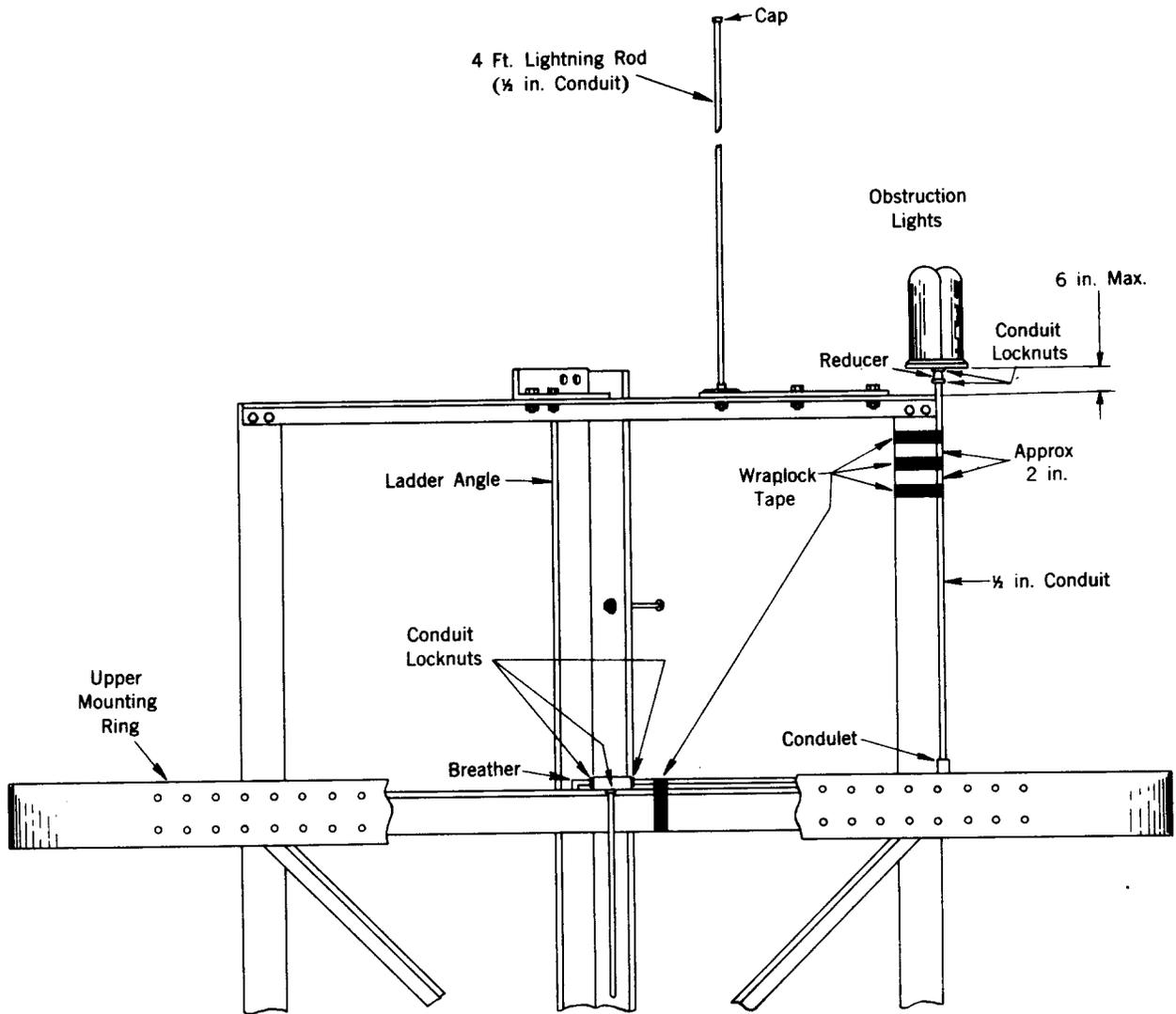
Fig. 2 - Dual 107-Watt Obstruction Lights — B Self-supporting Towers
