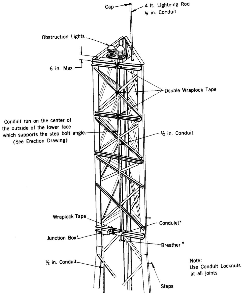
Fig. 2A - Dual 107-Watt Obstruction Lights - C Self-supporting Towers
