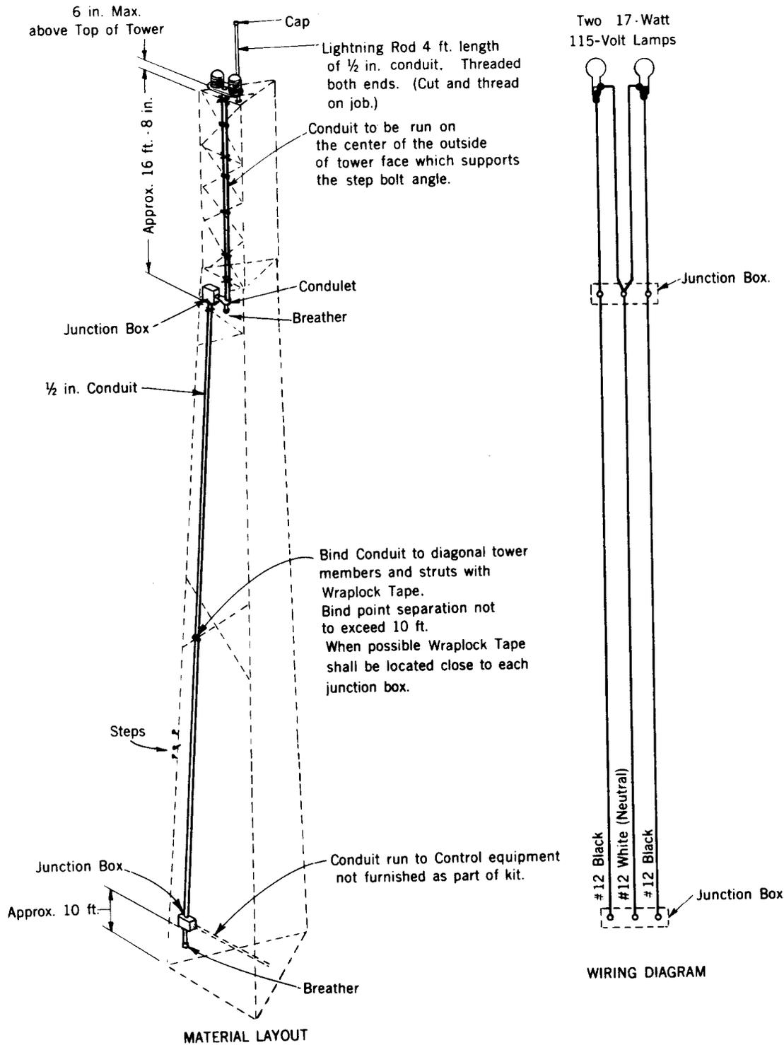
Fig. 5A - F.C.C. 17.24 Lighting - C Self-supporting Towers
