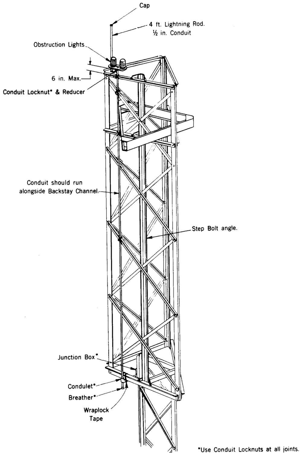
Fig. 3A - Dual 107-Watt Obstruction Lights - C Guyed Towers
