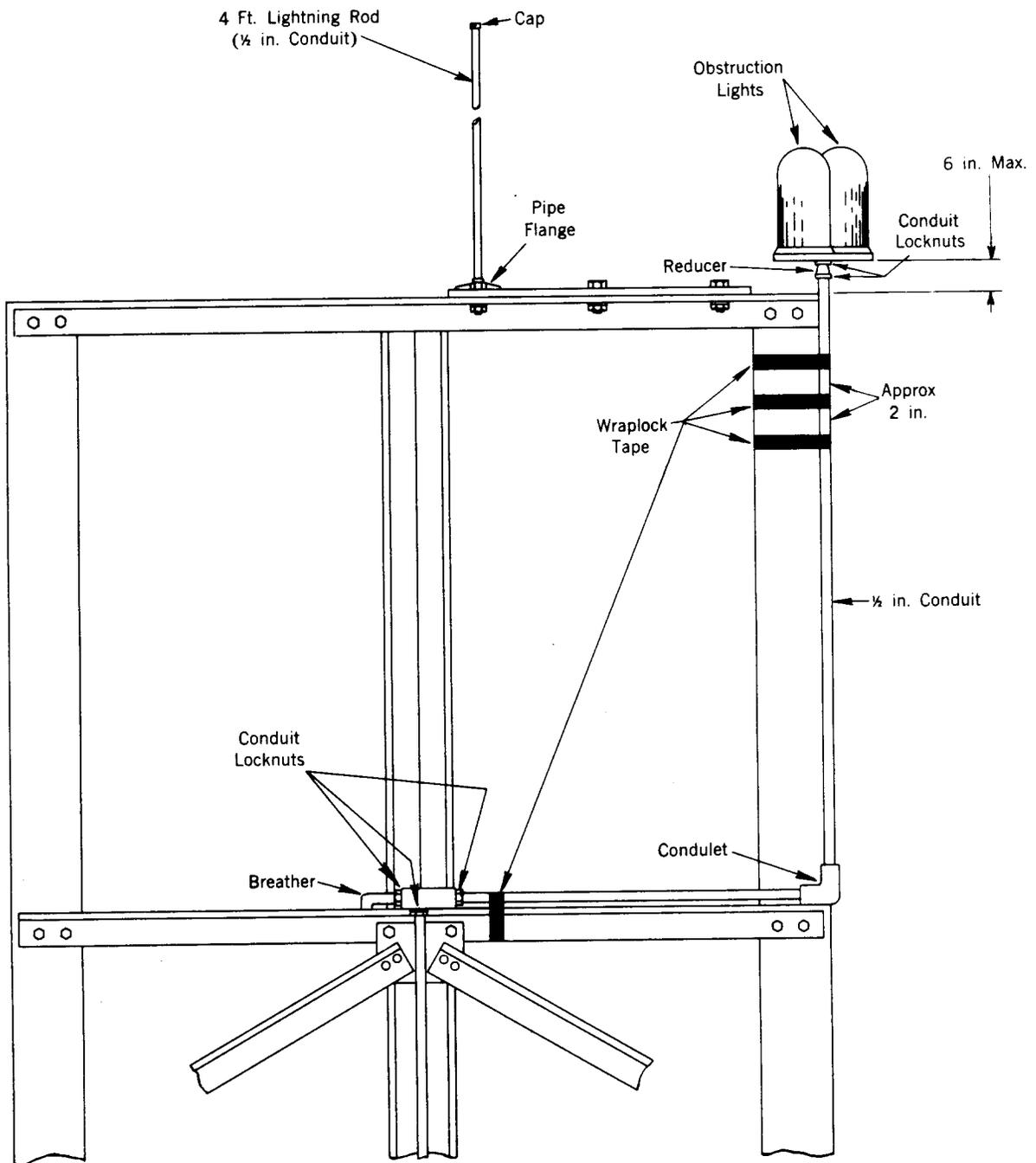
Fig. 3 - Dual 107-Watt Obstruction Lights - B Guyed Towers
