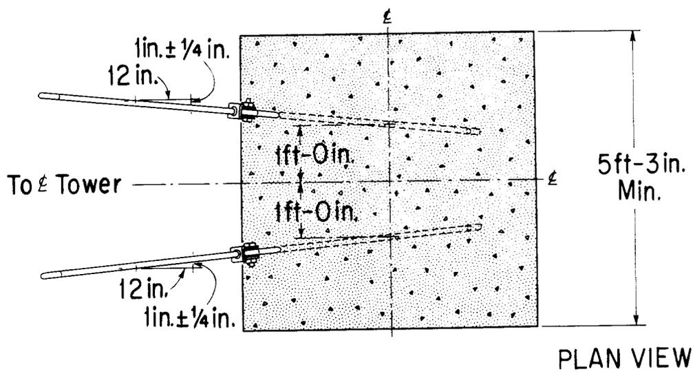
Fig. 5 - Anchor Used with 80 foot Tower
