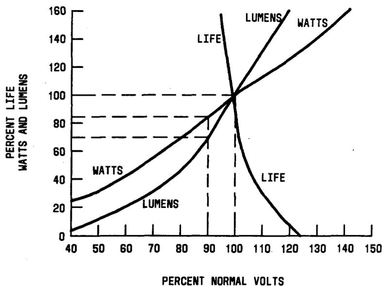
Fig. 1—Watts and Lumens
