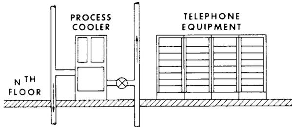
**Fig. 1—Horizontal System—Process Cooler Fed by Chiller on Same Floor**
