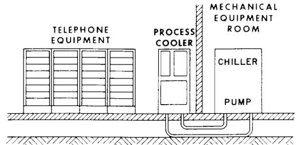
**Fig. 2—Vertical System—Process Coolers on Each Floor, All Fed by a Single Chiller**
