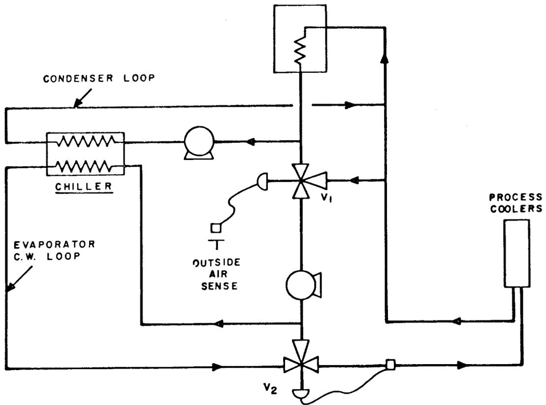
Fig. 9—Chiller Economizer System With Water-Glycol Loop
