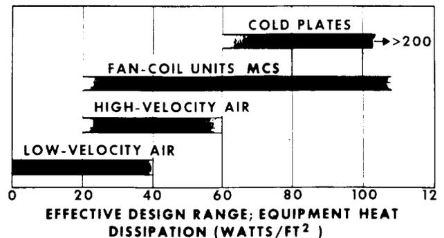
Fig. 3—As Heat Dissipation Increases for Contemporary Equipment, Cooling Systems Using Chilled Water Have Become More Economical Than All-Air Systems. The Effective Design Range of the New Modular Cooling System (MCS) Extends from Below 30 Watts/Ft<sup>2</sup> to More Than 100 Watts/Ft<sup>2</sup>
