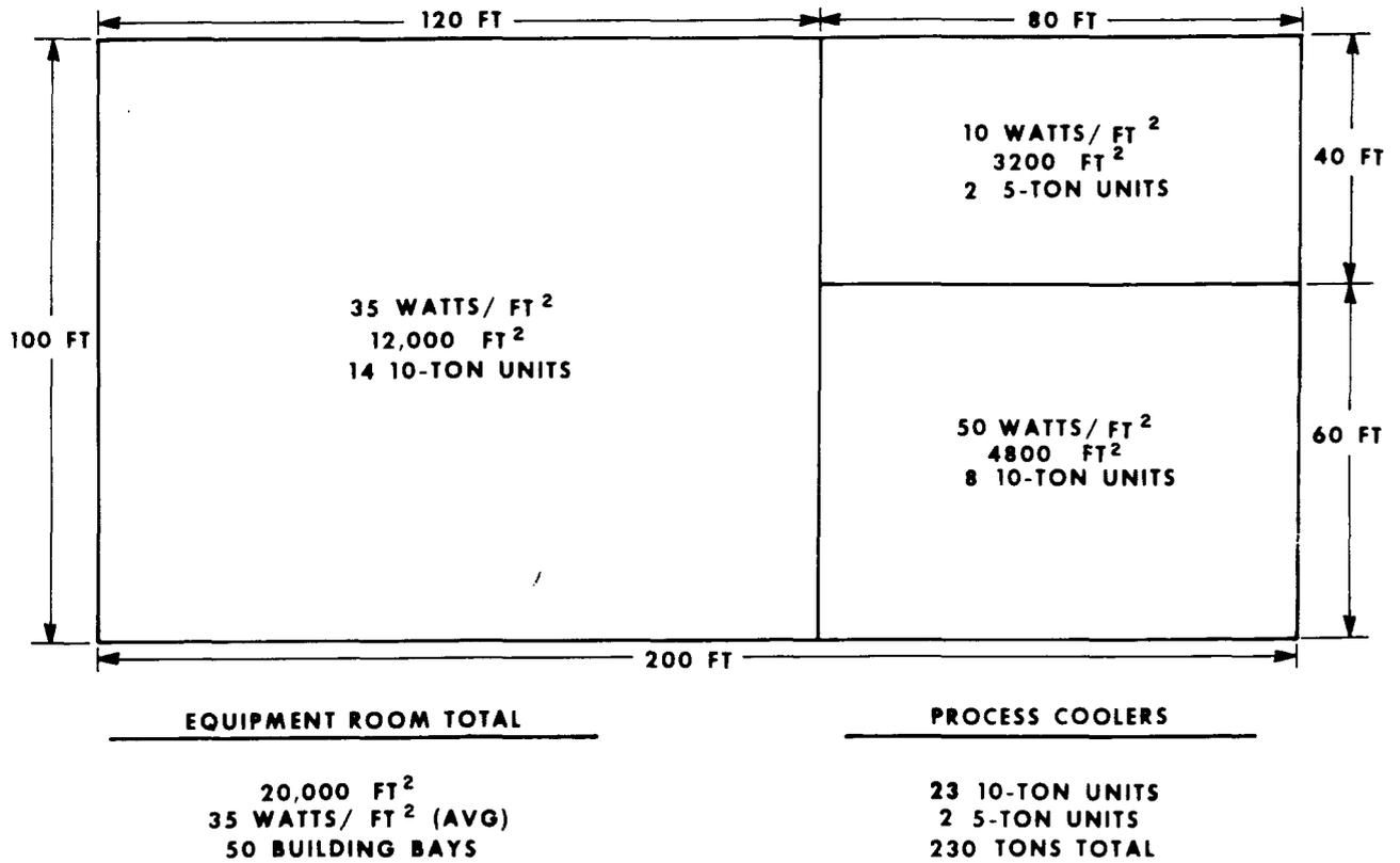
Fig. 10—The Equipment Heat Dissipation Pattern in a Hypothetical No. 4 ESS Installation Indicates an Average of Over 35 Watts/Ft<sup>2</sup>. Equipment Cooling Can Be Achieved With Twenty-three 10-Ton Process Coolers. Building Solar Load, Ventilation, Dehumidification, and Personnel Heat Loads Are in Addition to These Equipment and Lighting Loads
