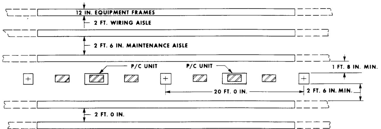
Fig. 6—Location of 5-Ton Process Coolers on Standard Floor Plan
