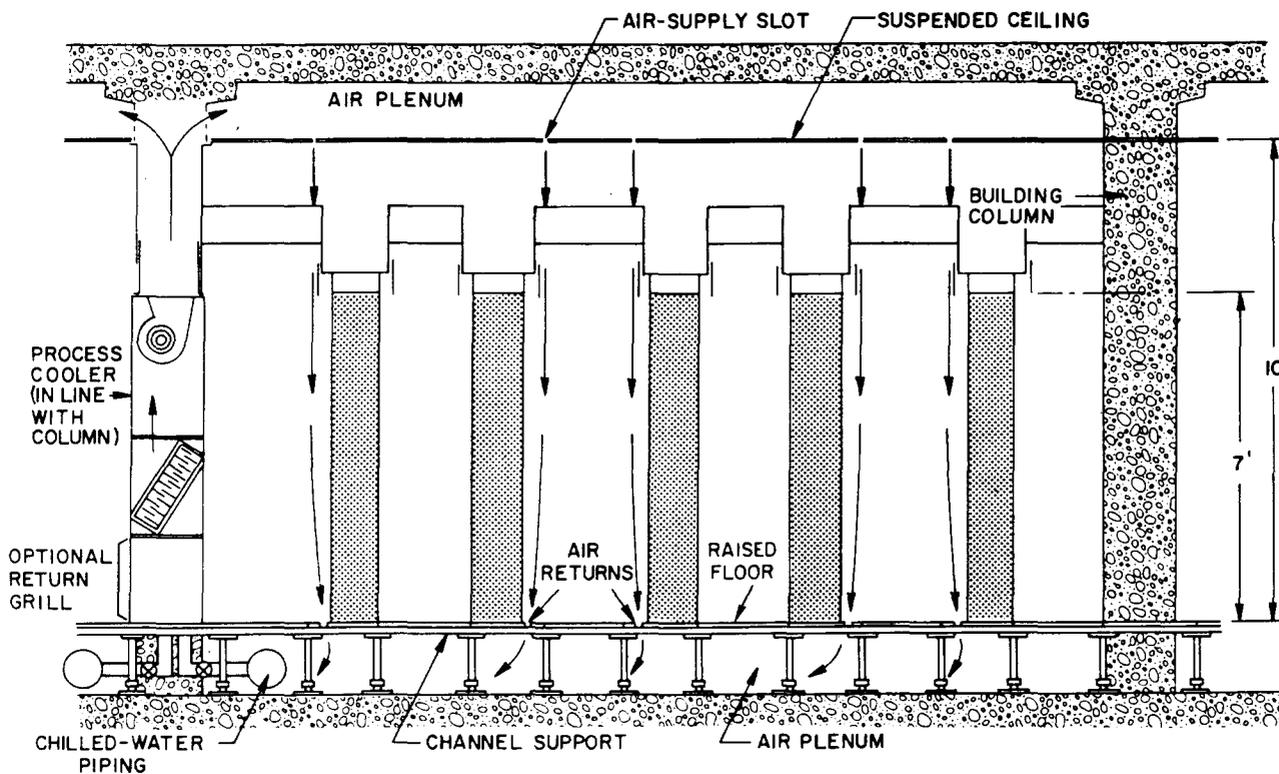
Fig. 7—Modular Cooling System, 20-Foot by 20-Foot Building Bay Elevation Air Distribution. Arrows Show the Direction of the Airflow
