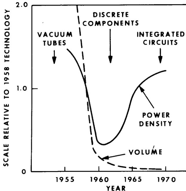
Fig. 2—Increases in Power Density of Data Processing Type Equipment Have Created Heat Transfer Problems that Require New Cooling Methods
