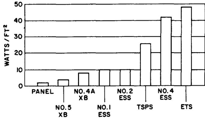
Fig. 1—Heat (Average) Dissipated by Telephone Equipment Has Increased from Less Than 10 Watts/Ft<sup>2</sup> for Electromechanical Equipment to Over 40 Watts/Ft<sup>2</sup> for the New Toll Electronic Switching Systems
