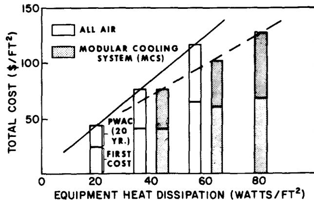
Fig. 4—Estimates of the Total Cost of Heat Removal per Square Foot Indicate a 20-Year PWAC (Taxes, Operation, and Maintenance) Which Is Comparable to the First Class (Air-Conditioning System and Building Space). The MCS Shows Economies at Equipment Heat Loads Above 20 to 30 Watts/Ft<sup>2</sup>
