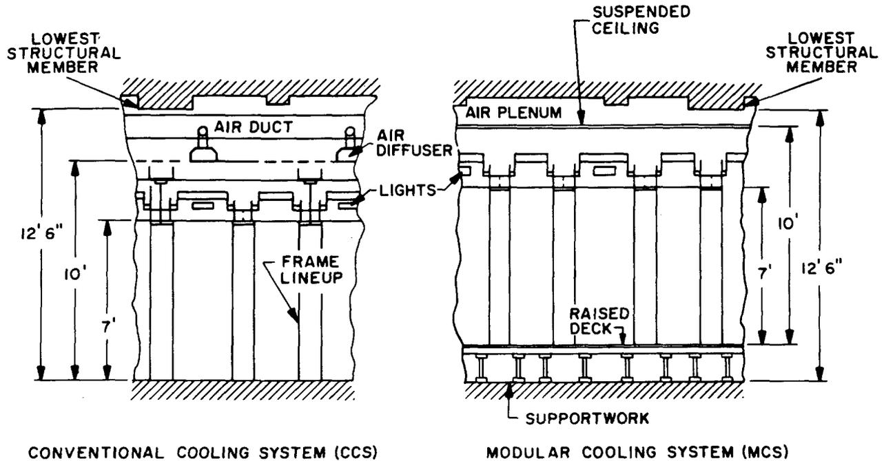
Fig. 5—The MCS includes Process Coolers Connected to a Ceiling Air Plenum Supply, to a Floor Air Return Plenum, and to Chilled-Water Distribution Under a Raised Deck. Conventional Cooling Is Achieved With an Overhead Supply and Return Duct System With Fans in a Remote Mechanical-Equipment Room
