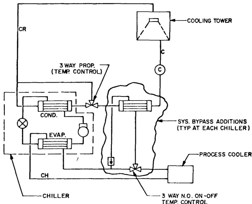
ROOM TEMPERATURE CAN BE MAINTAINED AT 80° F. BY BYPASS SYSTEM WHEN OUTSIDE WET BULB TEMPERATURE  $\leq$  35° F. PARTIAL LOAD COOLING CAPABILITY AT HIGHER TEMPERATURES.
