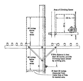
4.04 If the only supply conductors at a level above telephone cables, conductors, etc., are secondaries (0-750 volts between conductors) supplying airport or airway marker lights, or crossing over the telephone line and attached to the pole top or to a pole top extension fixture, the width of the climbing space measured across the line may be reduced to 16 inches.
