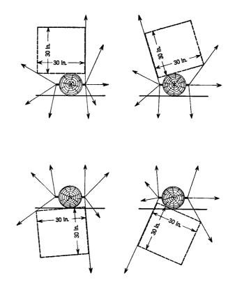
4.06 Where climbing space cannot otherwise be obtained on either the field or street side of the pole, place a guard arm and distribute from it, or place span clamps on the suspension strand.
