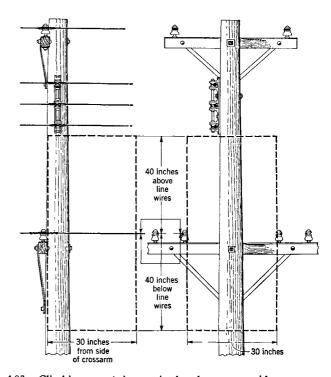
4.03 Climbing space is required only on one side or corner of the pole. Portions of the pole when included in one side or corner of the climbing space, and vertical runs incased in conduit (or other protective covering) and securely attached to the surface of the pole are not considered to obstruct the climbing space.
