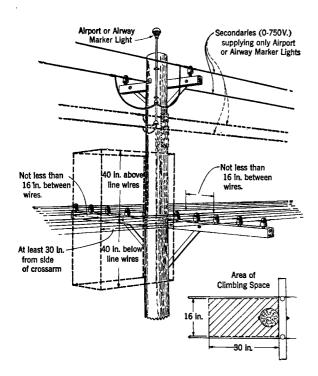
4.05 When drop wire fixtures are attached directly to a jointly used pole, distribute from the face or back of the pole. Examples of how climbing space should be measured in typical cases of drop wire distribution are shown in the following illustrations.
