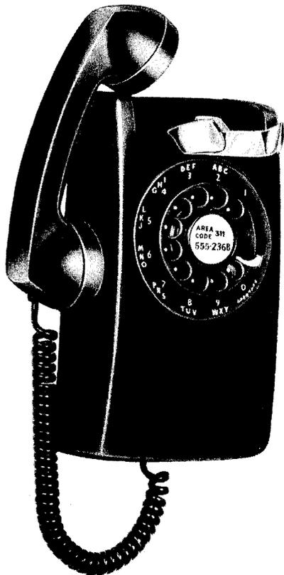
Fig. 9 — 554- or 556-Type Telephone Set, Handset Rest Position
