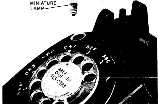
Fig. 28 — Lamp Assembly, 500H/P Telephone Sets
