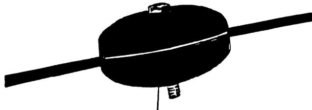
TIGHTEN WITH 7/16 IN. WRENCH (DO NOT USE 216 TYPE TOOL)
