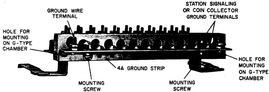
**Fig. 6—Installation of 4-Type Ground Strip**
