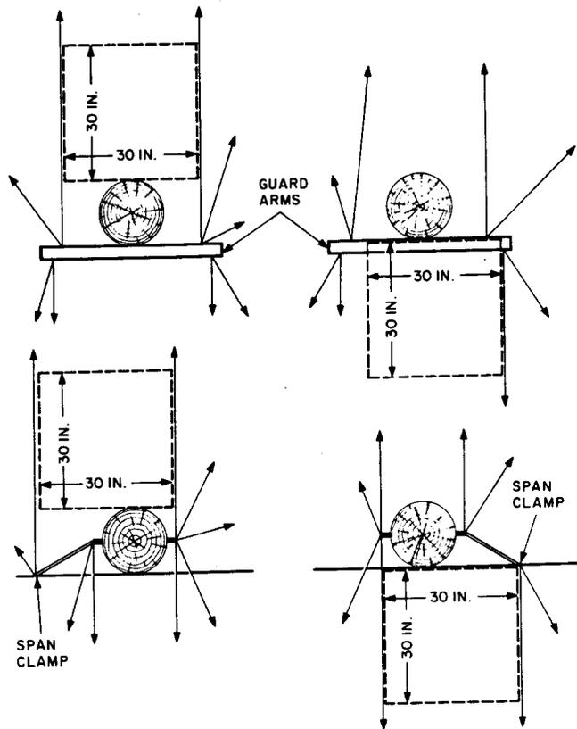
Fig. 5—Use of Guard Arm or Span Clamp to Maintain Climbing Space
