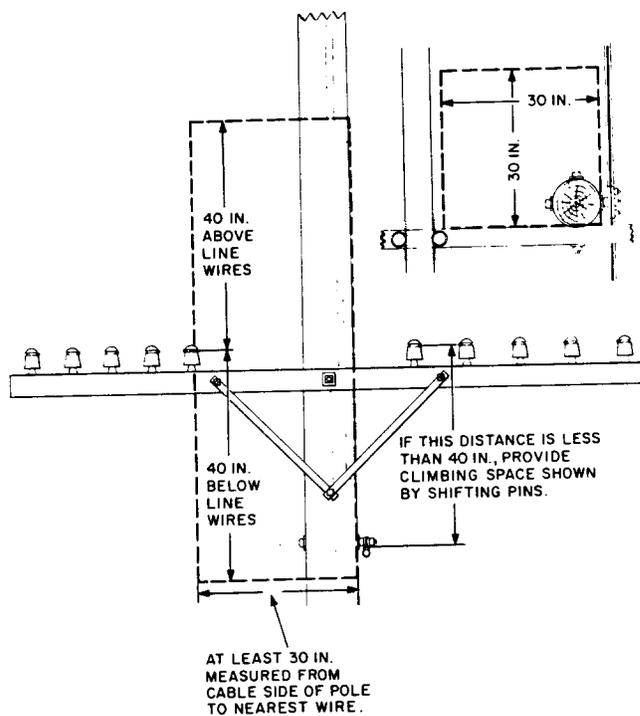
Fig. 6—Respacing Pins for Climbing Space
