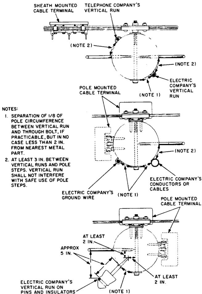
Fig. 1—Typical Vertical Run Clearances
