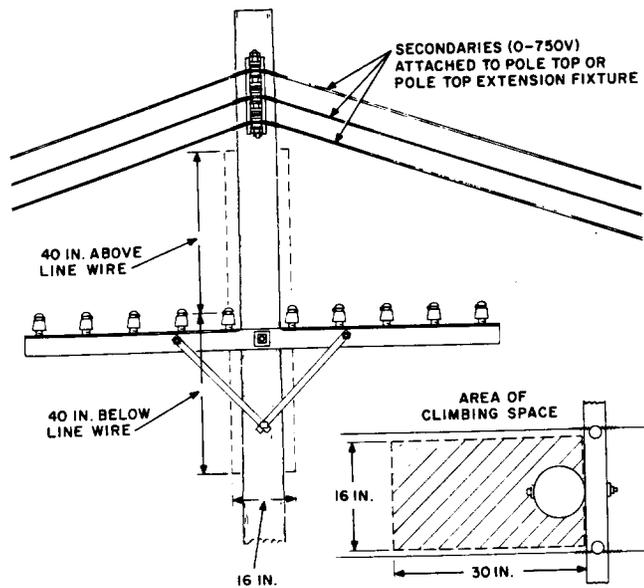
Fig. 3—Secondary Feeder Crossing Over Telephone Lines
