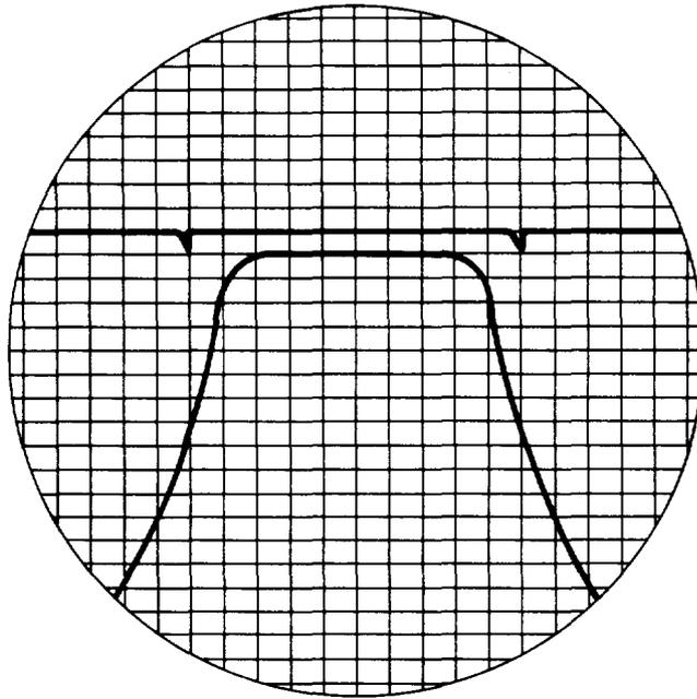
**Fig. 2—Typical Response of RF Amplifier and Mixer IF Pre-amplifier Stages**
