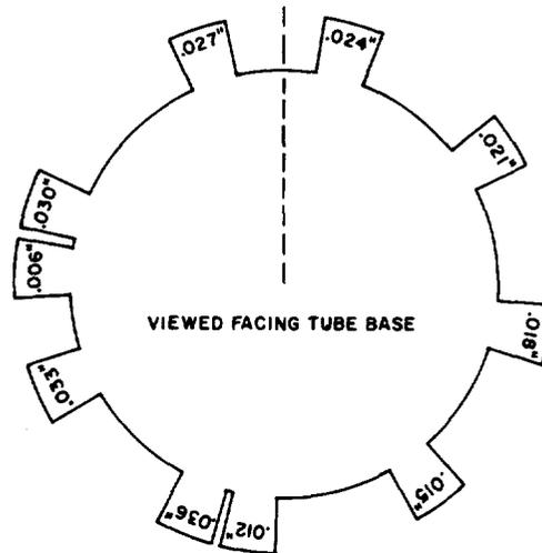
METHOD OF OBTAINING ANGULAR ALIGNMENT
