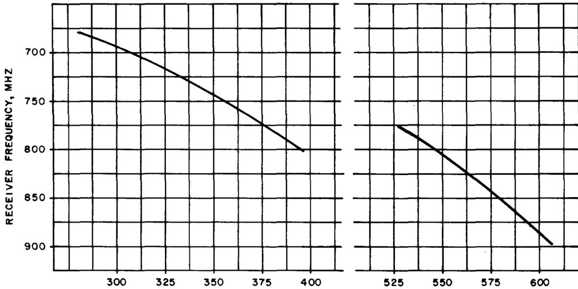
Fig. 1—Output Cavity—Tuning Control Setting
