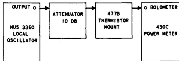
Fig. 2—Local Oscillator Output Power Measurement—Test Setup Diagram
