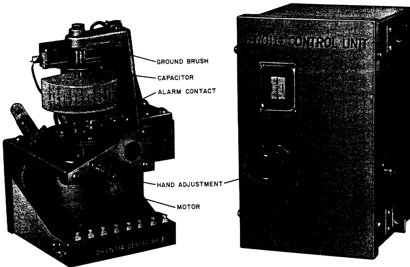
Fig. 1—50-A Automatic Frequency Control Unit
