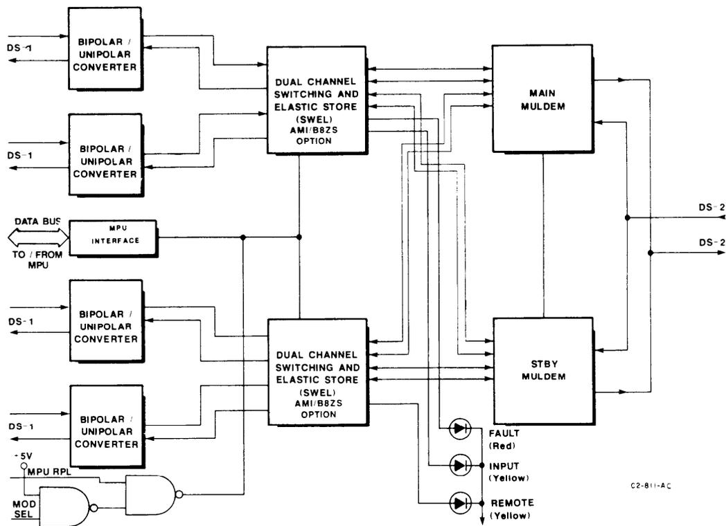
Figure 2A-3. LS INTER T1 Card Block Diagram
