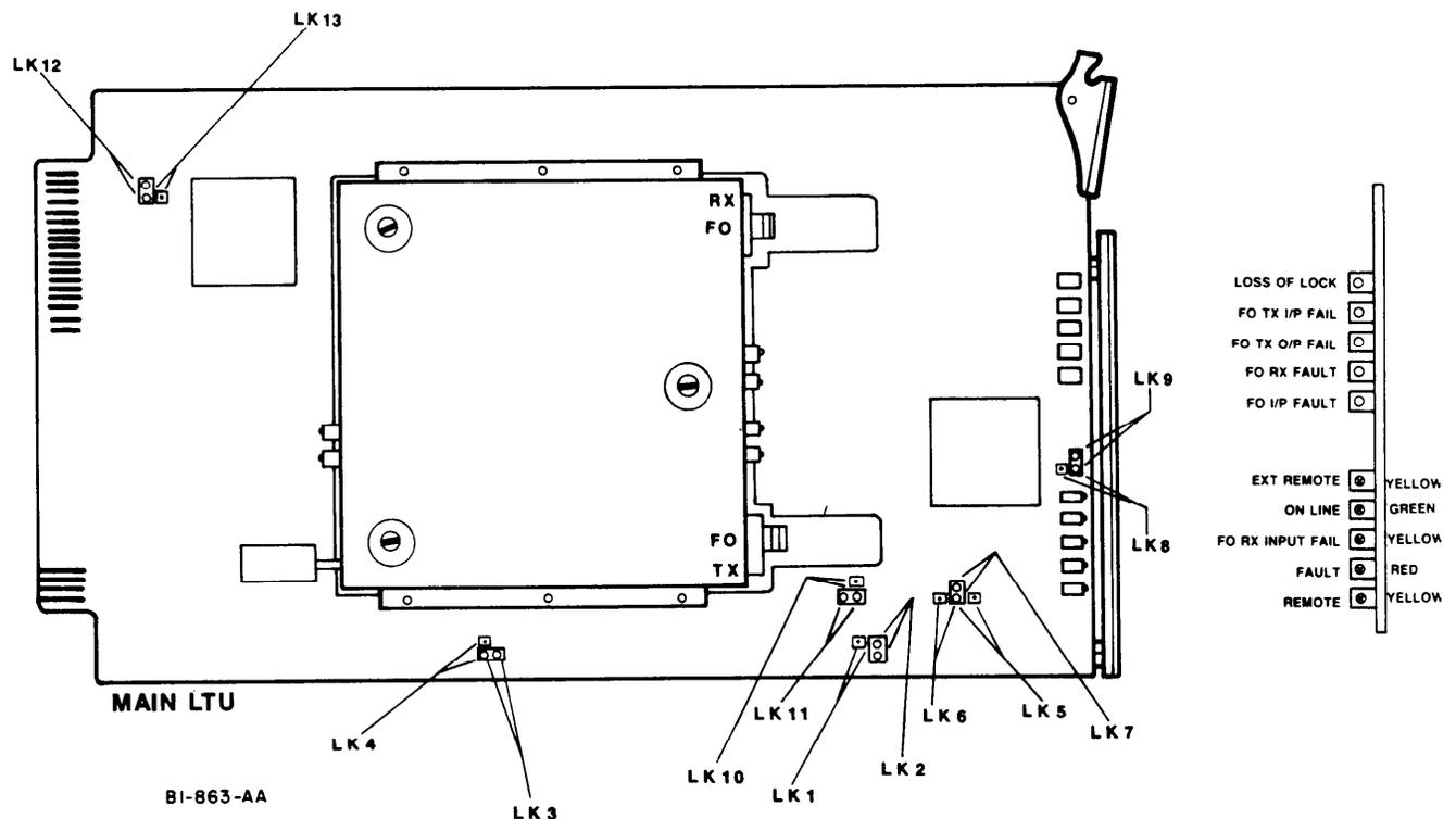
Figure 2C-1. LTU Low-Speed Interface Card (MAIN LTU illustrated)
