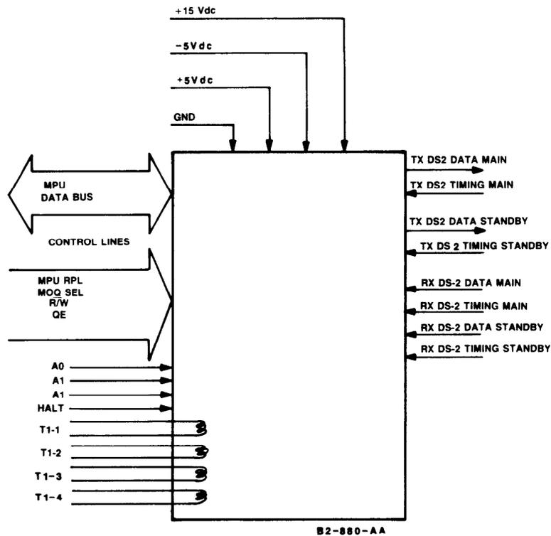
Figure 2A-2. LS INTER T1/T1C Card Interfaces
