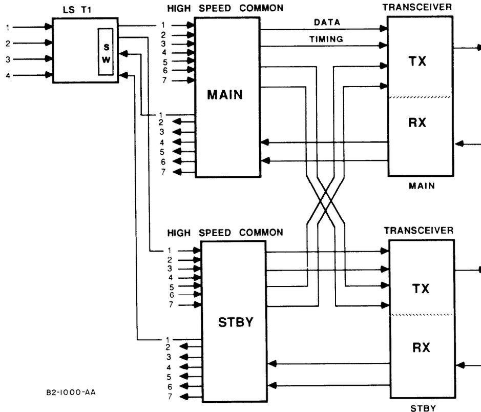
Figure 2-2. 828AF Digital Multiplexer Block Diagram
