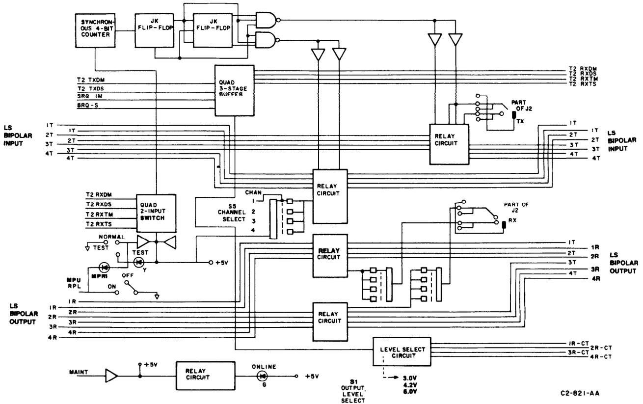
Figure 2-6. Maintenance Interface Card Block Diagram
