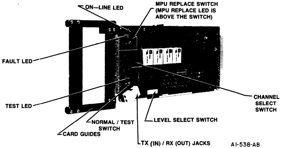
Figure 2-5. Maintenance Interface Card
