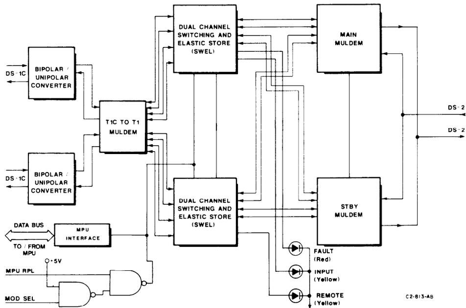
Figure 2A-4. LS INTER T1C Card Block Diagram
