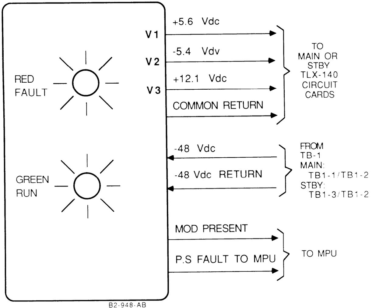
Figure 2H-2. PS Module Interfaces
