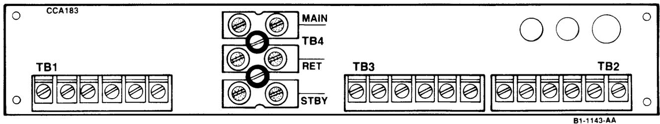
Figure 2-4. ACX043 Fuse and Alarm Panel
