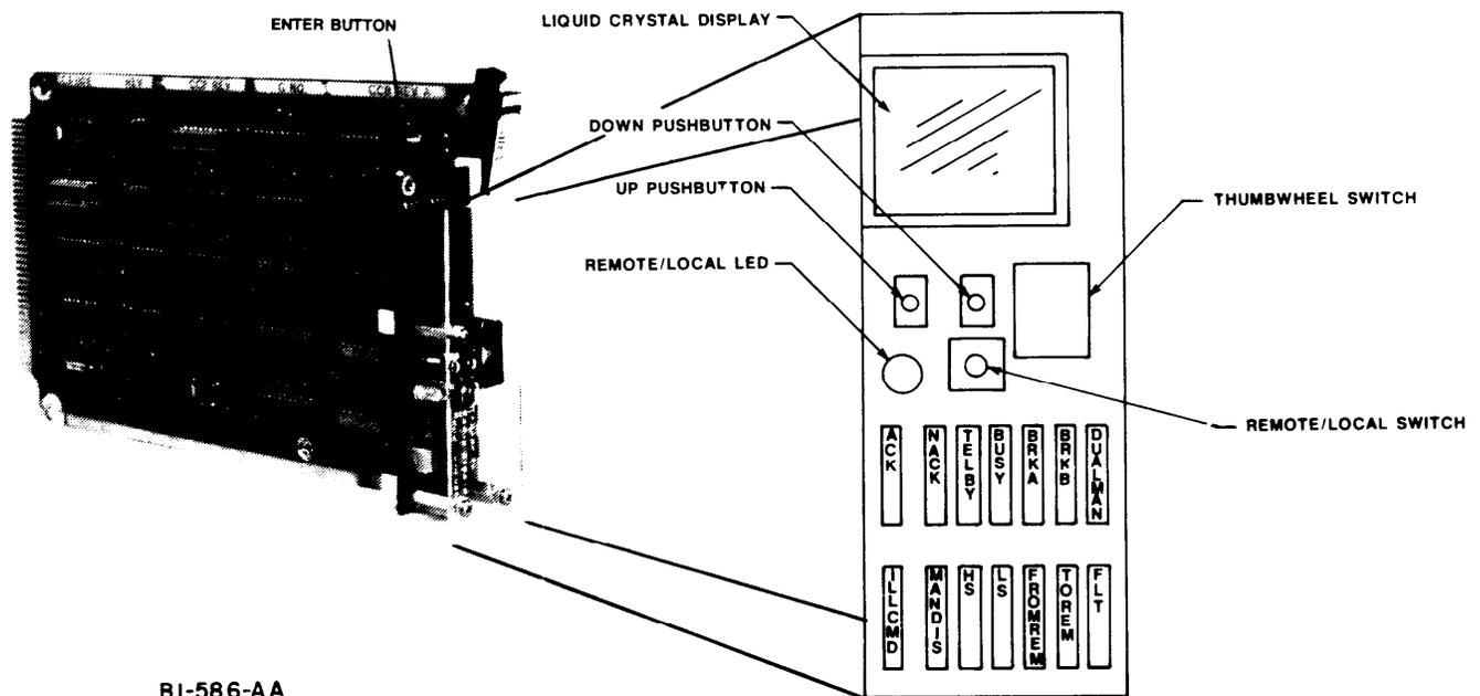
Figure 2-7. Manual Control Interface Card
