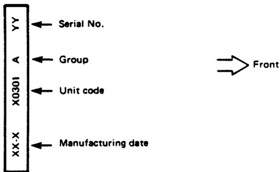
NOTE: Printed on the right side surface of the main board connector.
